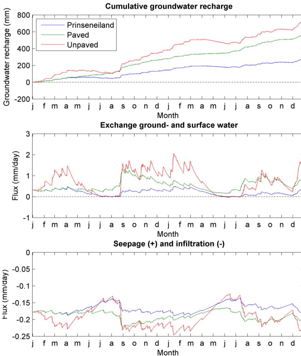
Figure 6.6. The simulated groundwater recharge, the flow of water between the urban ground- and the regional surface water and the flow between the urban and regional groundwater bodies over the years 2010 and 2011 for the Prinseneiland and a completely unpaved (green) and a completely paved Prinseneiland (red).
