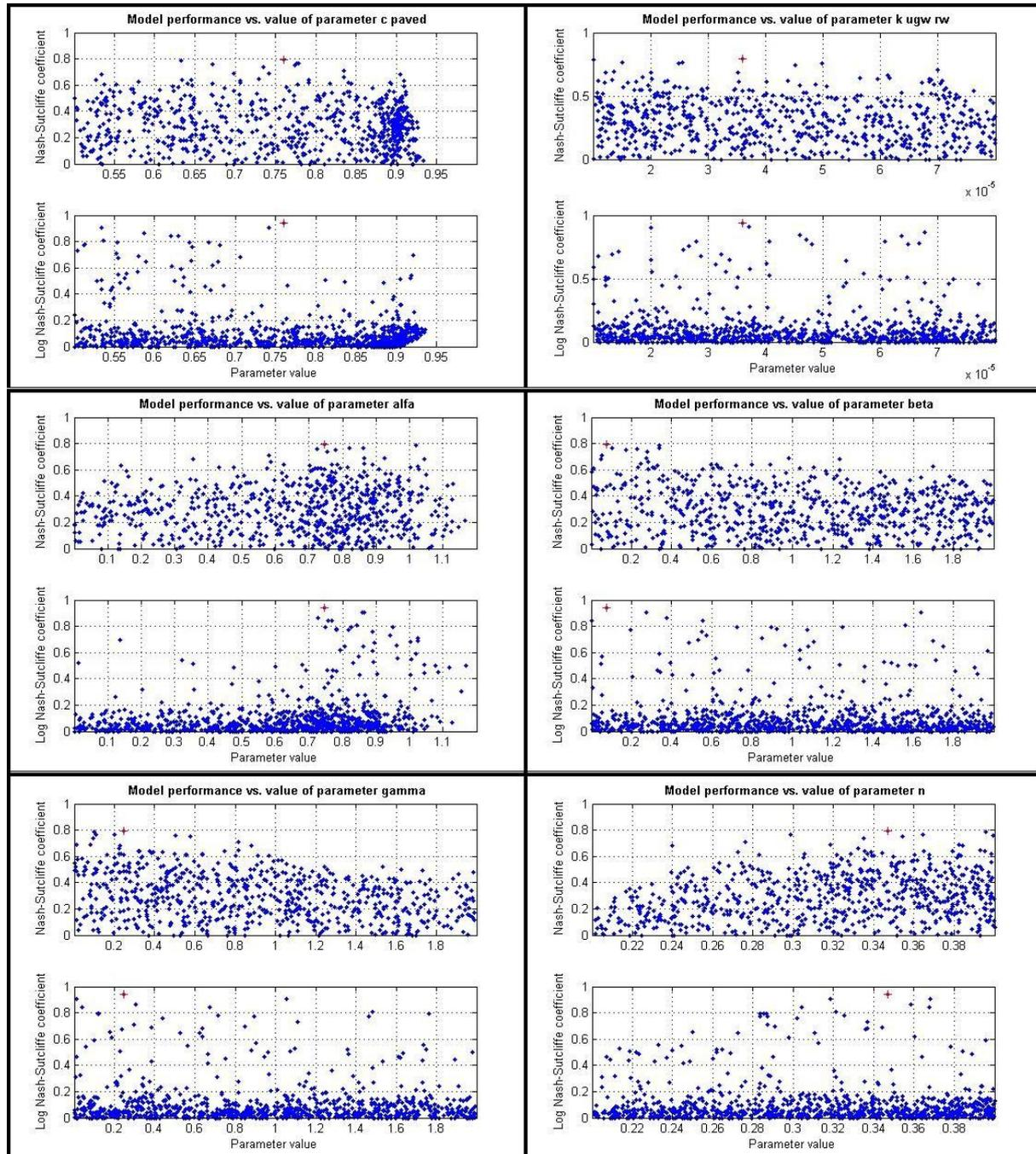
Figure 12.1. Performance of the model as a function of the values of the model parameters. The performance of the model is plotted vs. the values of 'c\_paved' (top left pair), 'k\_ugw\_rw' (top right pair), 'alfa' (middle left), 'beta' (middle right), 'gamma' (bottom left) and 'n' (bottom right). Each blue dot corresponds with the results of one Monte-Carlo run. The red cross indicates the calculated optimal parameter value.
