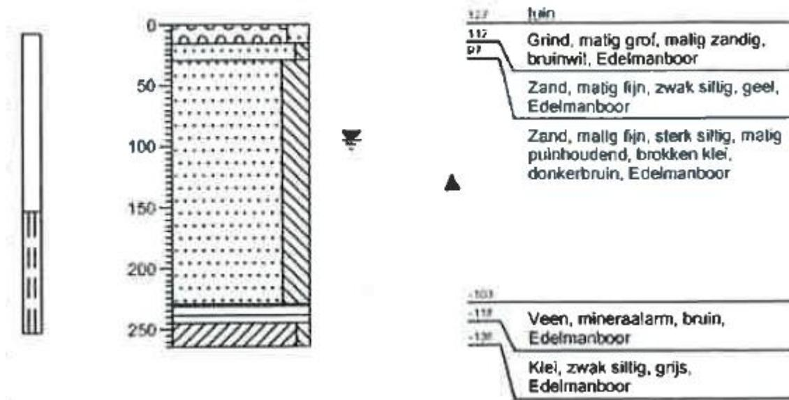
Figure 14.2. Soil survey on the location of piezometer C05268
