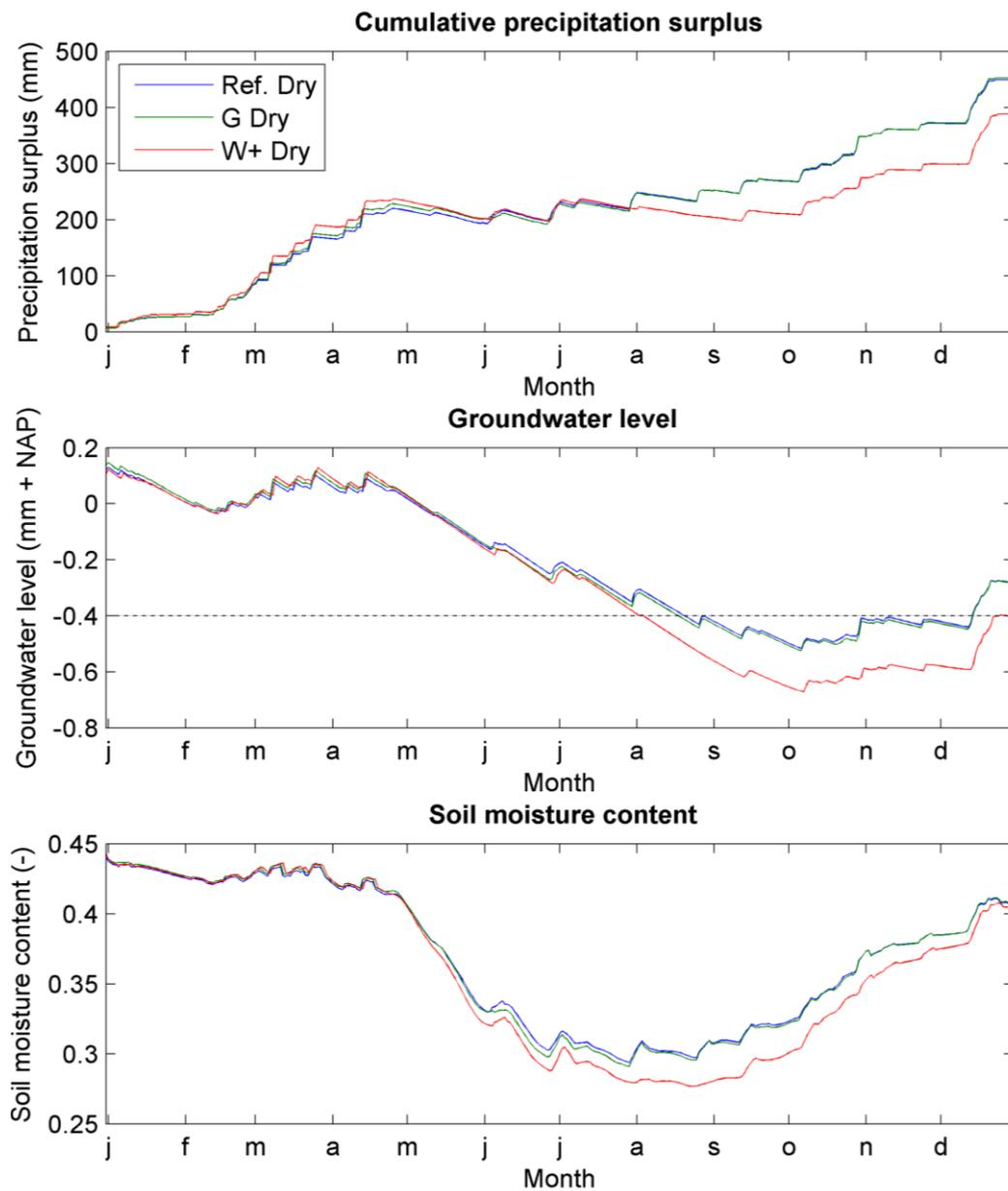
Figure 13.4. The simulated cumulative precipitation surplus (precipitation - evaporation), groundwater levels and soil moisture content over the 'Dry' years of the 'Reference' (blue line), 'G' (green) and 'W+' (red) climate scenarios for the Prinseneiland. The dotted line in the middle graph indicates the surface water level.
