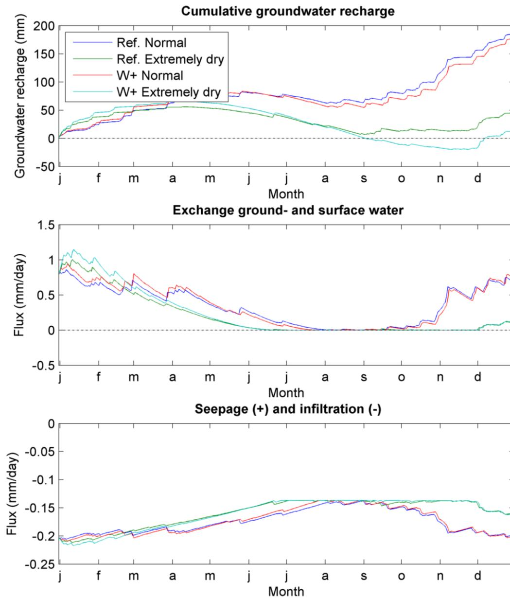
Figure 8.3. The simulated groundwater recharge, the flow of water between the urban ground- and the regional surface water and the flow between the urban and regional groundwater bodies over the scenario years 'Reference, Normal' (blue line), 'Reference, Extremely dry' (green), 'W+, Normal' (red) and 'W+, Extremely Dry' (cyan) for the Prinseneiland.
