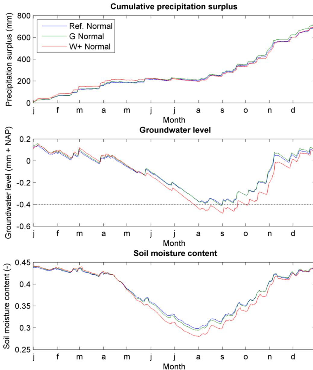
Figure 13.1. The simulated cumulative precipitation surplus (precipitation - evaporation), groundwater levels and soil moisture content over the 'Normal' years of the 'Reference' (blue line), 'G' (green) and 'W+' (red) climate scenarios for the Prinseneiland. The dotted line in the middle graph indicates the surface water level.
