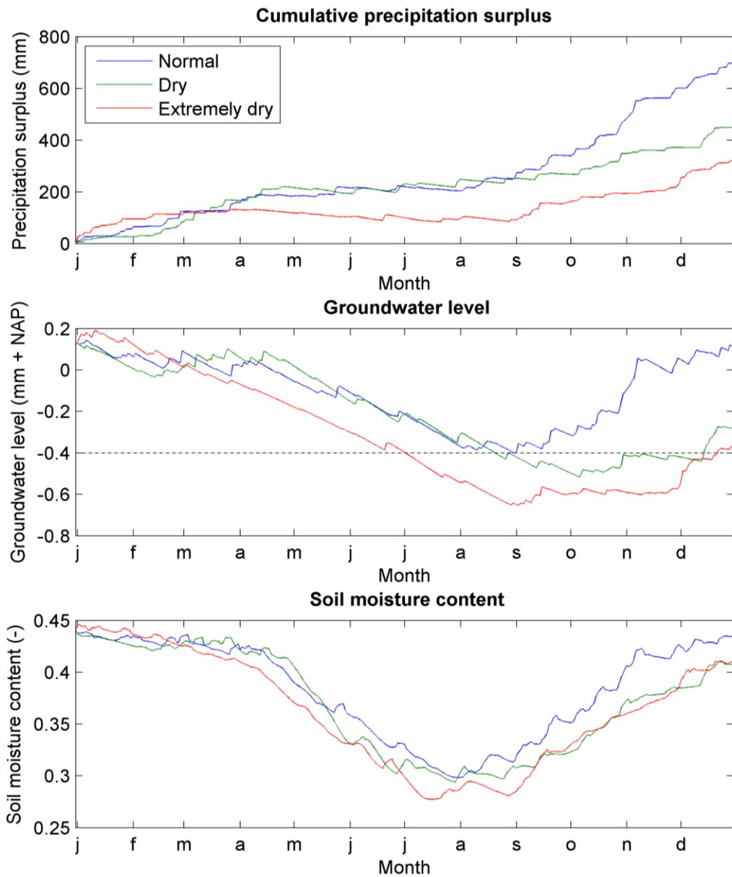
Figure 6.8. The simulated cumulative precipitation surplus (precipitation - evaporation), groundwater levels and soil moisture content over the scenario years 'Normal' (blue line), 'Dry' (green) and 'Extremely dry' (red) for the Prinseneiland. The dotted line in the middle graph indicates the surface water level.
