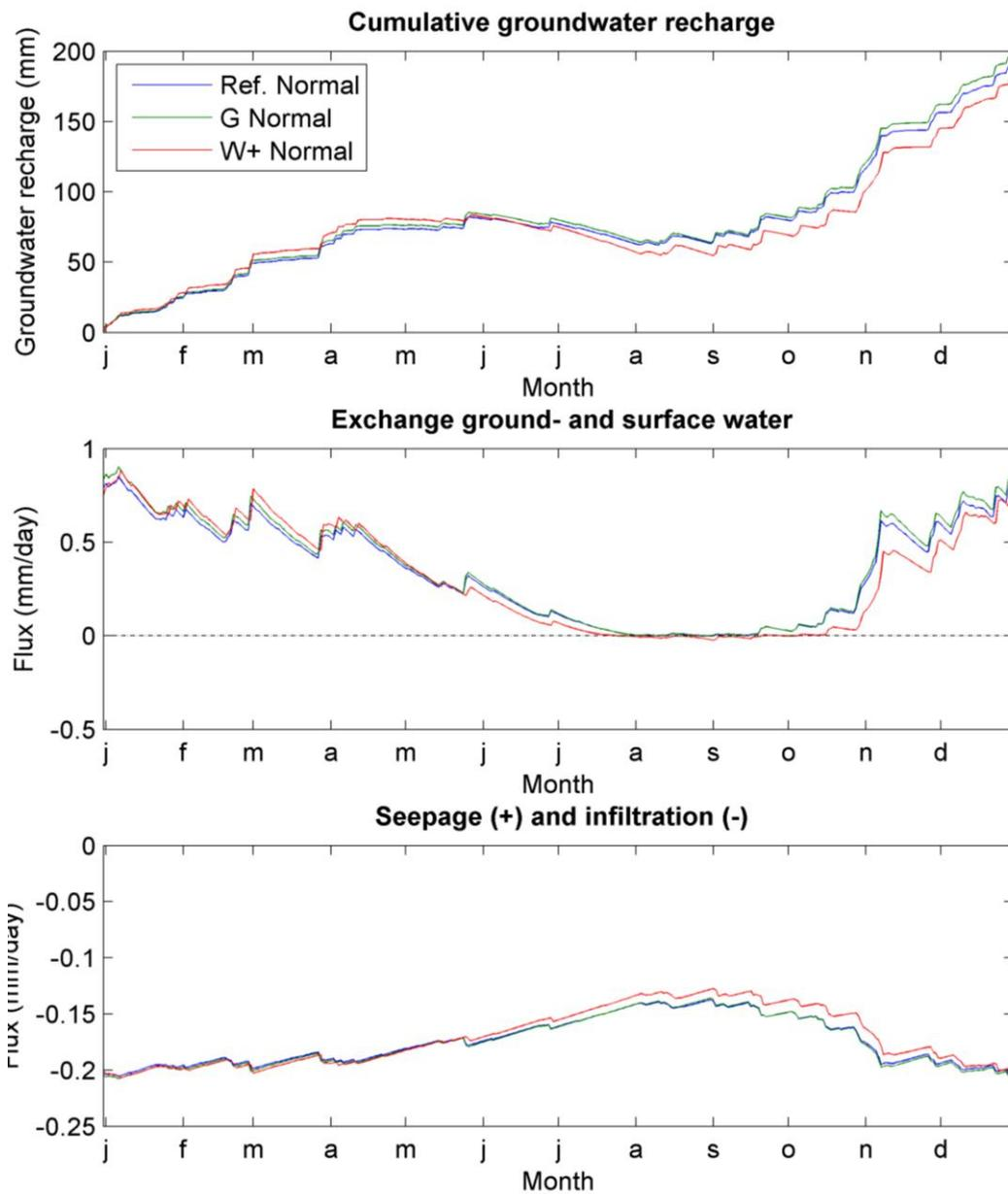
Figure 13.2. The simulated groundwater recharge, the flow of water between the urban ground- and the regional surface water and the flow between the urban and regional groundwater bodies over the 'Normal' years of the 'Reference' (blue line), 'G' (green) and 'W+' (red) climate scenarios for the Prinseneiland.
