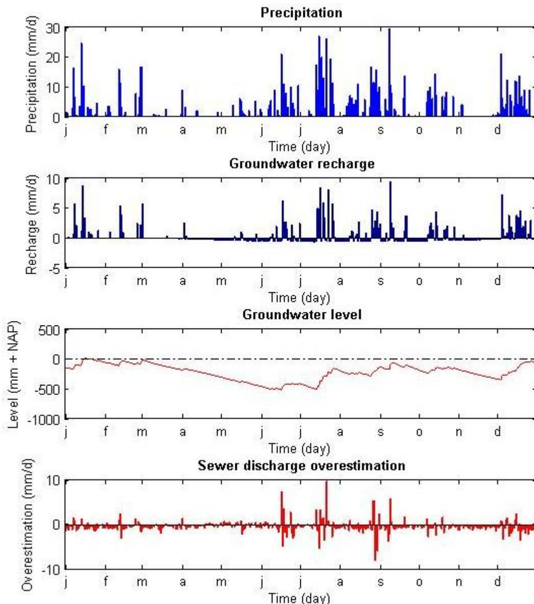
Figure 6.1. The main results of the model run for the Prinseneiland over the year 2011.
