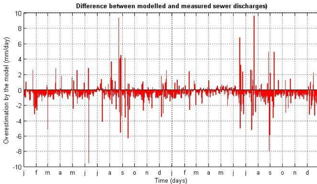
Figure 5.8. Difference between modelled and measured sewer discharges over the years 2010 and 2011. Positive values represent an overestimation by the model.
