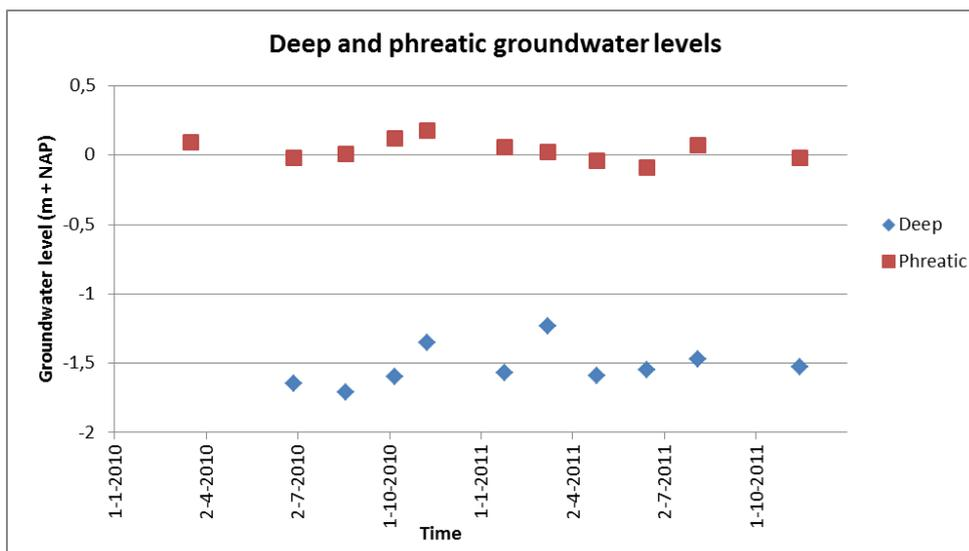
Figure 4.6. Groundwater levels over the years 2010 and 2011 in the Pleistocene sand layer (Deep) and the phreatic groundwater measured at the Galgenstraat.
