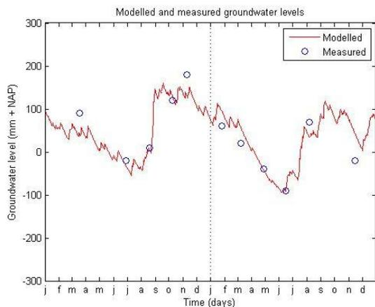
Figure 5.4. Simulated groundwater levels at the Galgenstraat with the optimal parameter values according to both performance indicators over the years 2010-2011.
