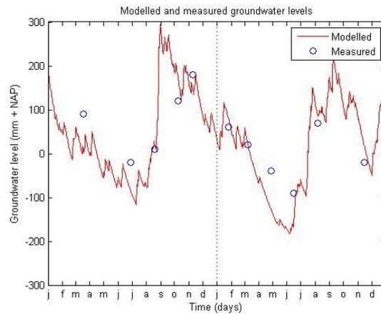
Figure 5.7. Simulated groundwater levels at the Galgenstraat with the optimal parameter values according to both performance indicators over the years 2010-2011.
