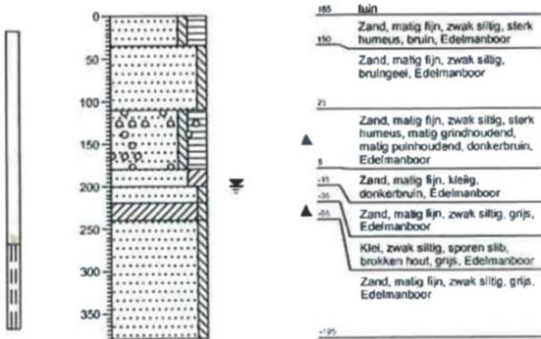
Figure 14.4. Soil survey on the location of piezometer C05270
