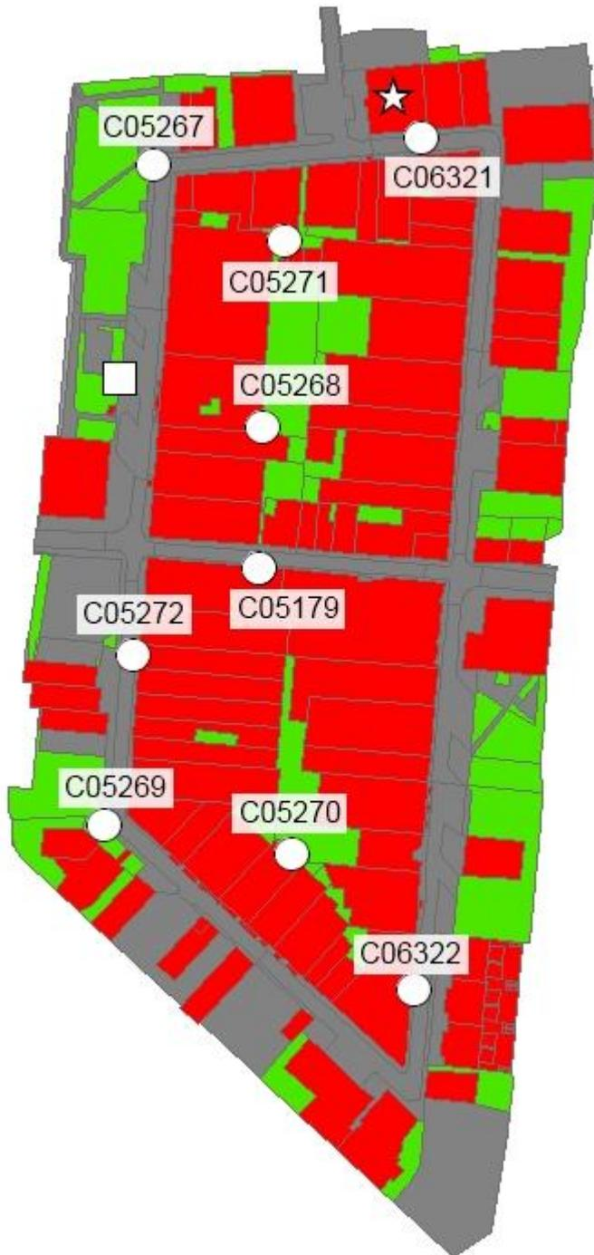
Figure 4.4. Locations of the piezometers, tipping bucket and sewer discharge measurements. The circles indicate the locations of the piezometers. The 'CO' numbers are the codes for the piezometers. The star specifies the location of the tipping bucket. The square indicates the location of the sewer pump on the island.
