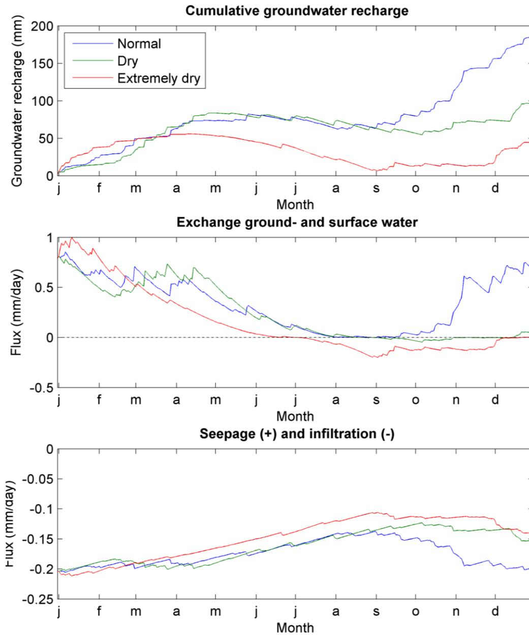
Figure 6.9. The simulated groundwater recharge, the flow of water between the urban ground- and the regional surface water and the flow between the urban and regional groundwater bodies over the scenario years 'Normal' (blue line), 'Dry' (green) and 'Extremely Dry' (red) for the Prinseneiland.
