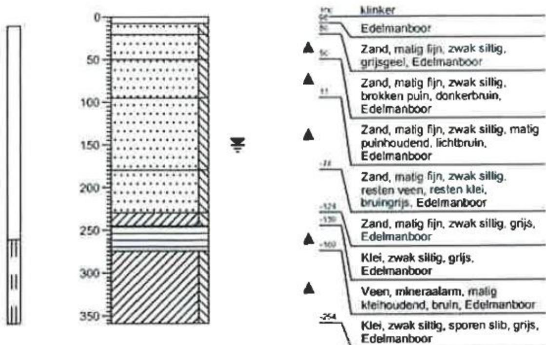
Figure 14.1. Soil survey on the location of piezometer C05267.
