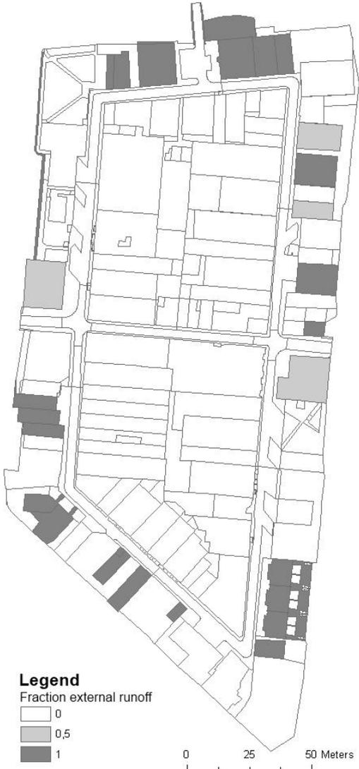
Figure 10.1. The fraction of precipitation on a feature being discharged outside the area boundaries.
