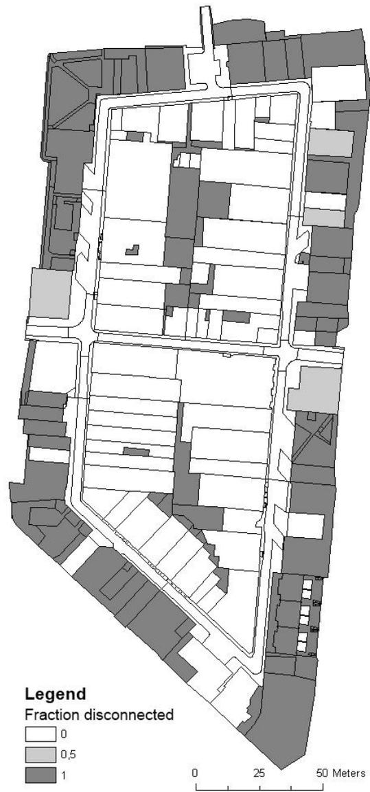
Figure 3.4. Assumed fraction of the precipitation on features not being discharged to a sewer.
