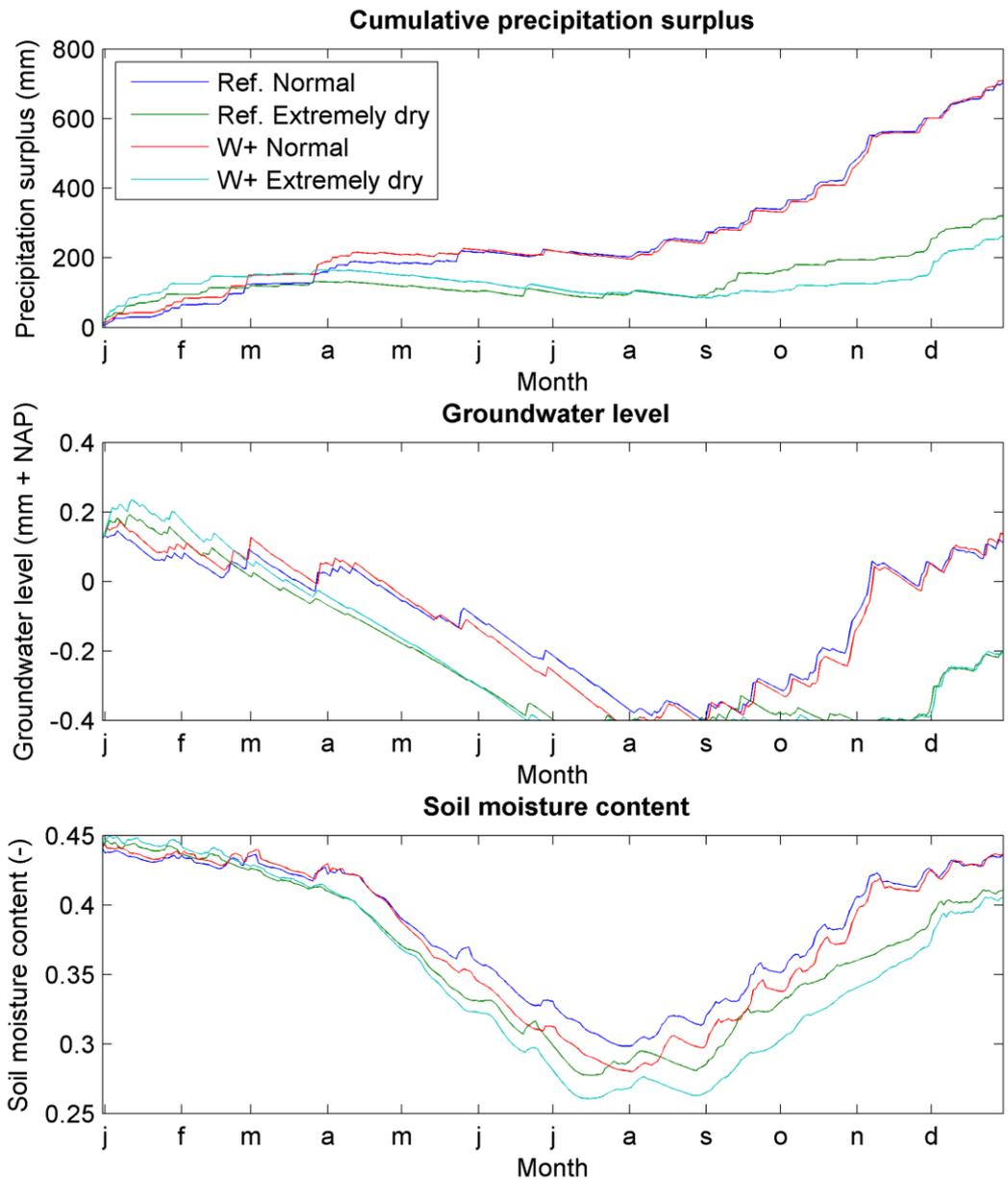
Figure 8.2. The simulated cumulative precipitation surplus (precipitation - evaporation), groundwater levels and soil moisture content over the scenario combinations 'Reference, Normal' (blue line), 'Reference, Extremely dry' (green), 'W+, Normal' (red) and 'W+, Extremely dry' (cyan) for the Prinseneiland. The dotted line in the middle graph indicates the surface water level.
