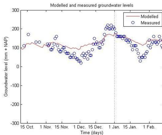
Figure 5.5. Simulated groundwater levels at the Galgenstraat with the optimal parameter values according to both performance indicators from Oct. 2012-Feb. 2013.
