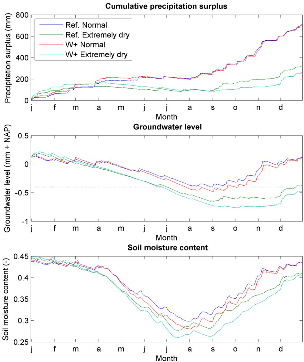
Figure 6.12. The simulated cumulative precipitation surplus (precipitation - evaporation), groundwater levels and soil moisture content over the scenario combinations 'Reference, Normal' (blue line), 'Reference, Extremely dry' (green), 'W+, Normal' (red) and 'W+, Extremely dry' (cyan) for the Prinseneiland. The dotted line in the middle graph indicates the surface water level.
