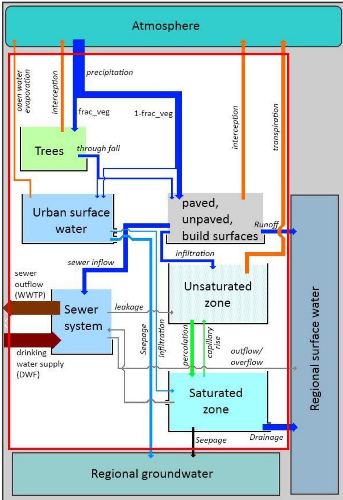
Figure 5.1. Structure of the model showing the storages and fluxes and some simplified relations. The thicknesses of the arrows are for illustrative purposes only. They should not be interpreted as the size of the fluxes. The red line indicates the model boundary.
