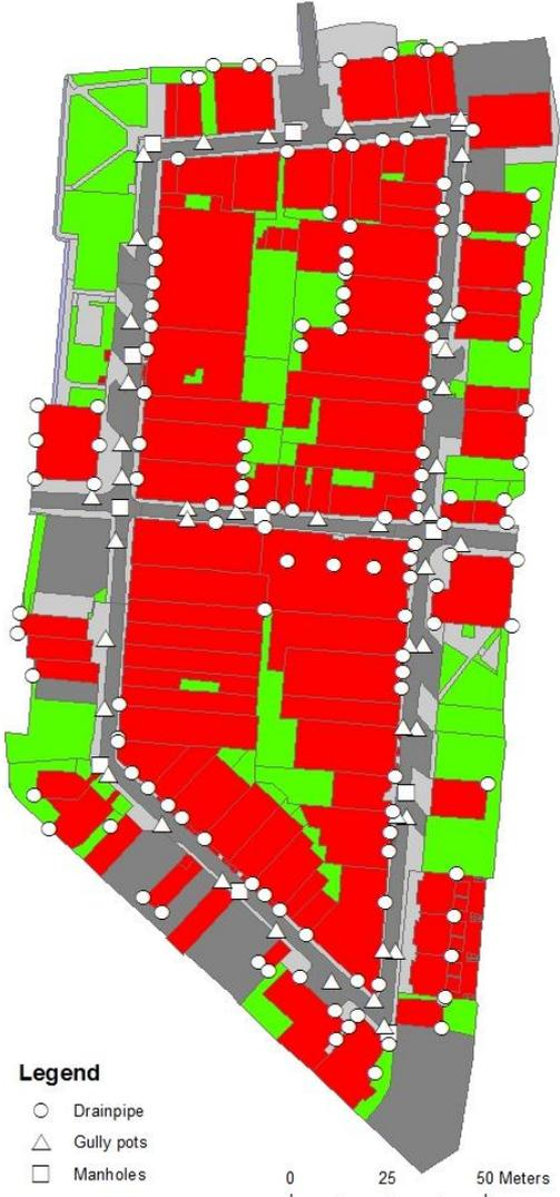
Figure 10.2. The locations of the drainpipes from the buildings, gully pots and manholes determined during the fieldwork. The red colour indicates the buildings on the island, whilst the grey shades denote the paved areas and the green the unpaved areas.
