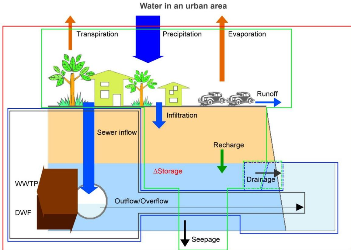
Figure 2.1. Schematisation of the urban water cycle (red box). The urban water cycle consists of the urban hydrological cycle (green box) and the urban water system (blue box). The small urban water cycle is shown in the dark grey box.
