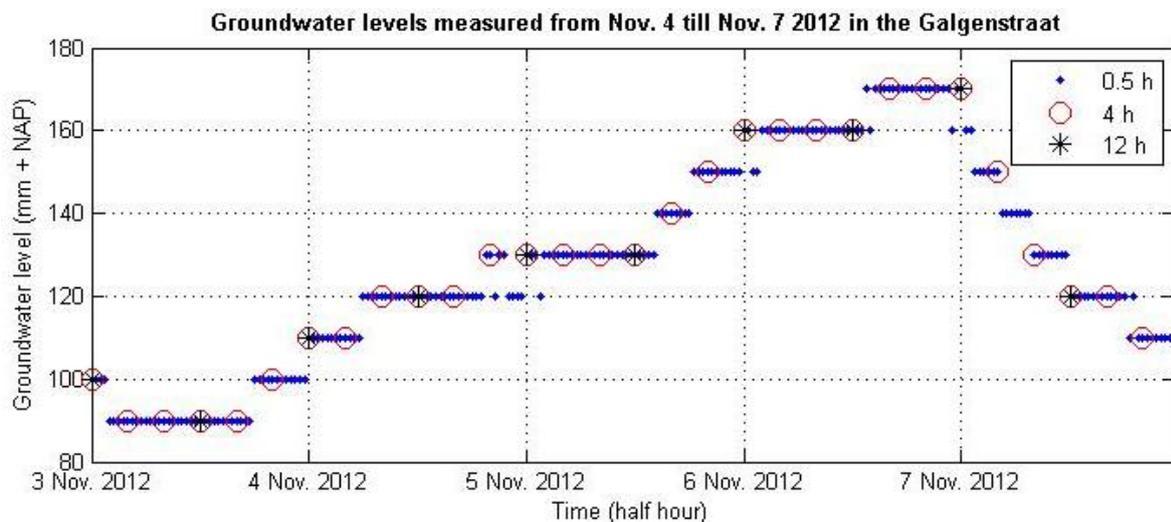
Figure 7.1. Groundwater level measurements from the 4<sup>th</sup> till the 7<sup>th</sup> of November 2012 in the Galgenstraat. The blue indicate the actual data. The red circle and black asterisk indicate hypothetical datasets for measurements with a lower frequency of once every 4 and 12 hours respectively.
