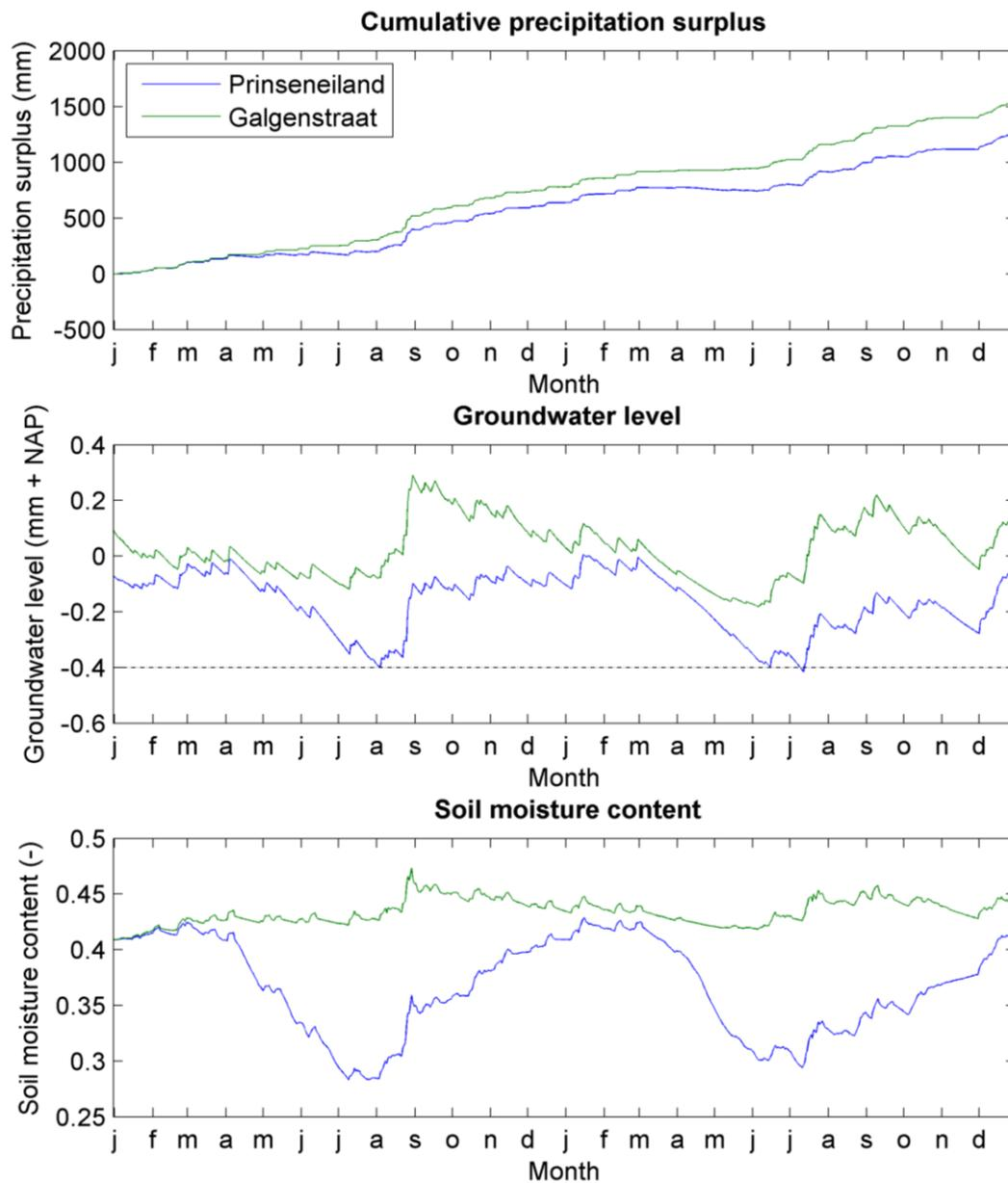
Figure 6.3. The simulated cumulative precipitation surplus (precipitation - evaporation), groundwater levels and soil moisture content over the years 2010 and 2011 for the entire Prinseneiland (blue) and at the measuring point at the Galgenstraat (green). The dotted line in the middle graph indicates the surface water level.
