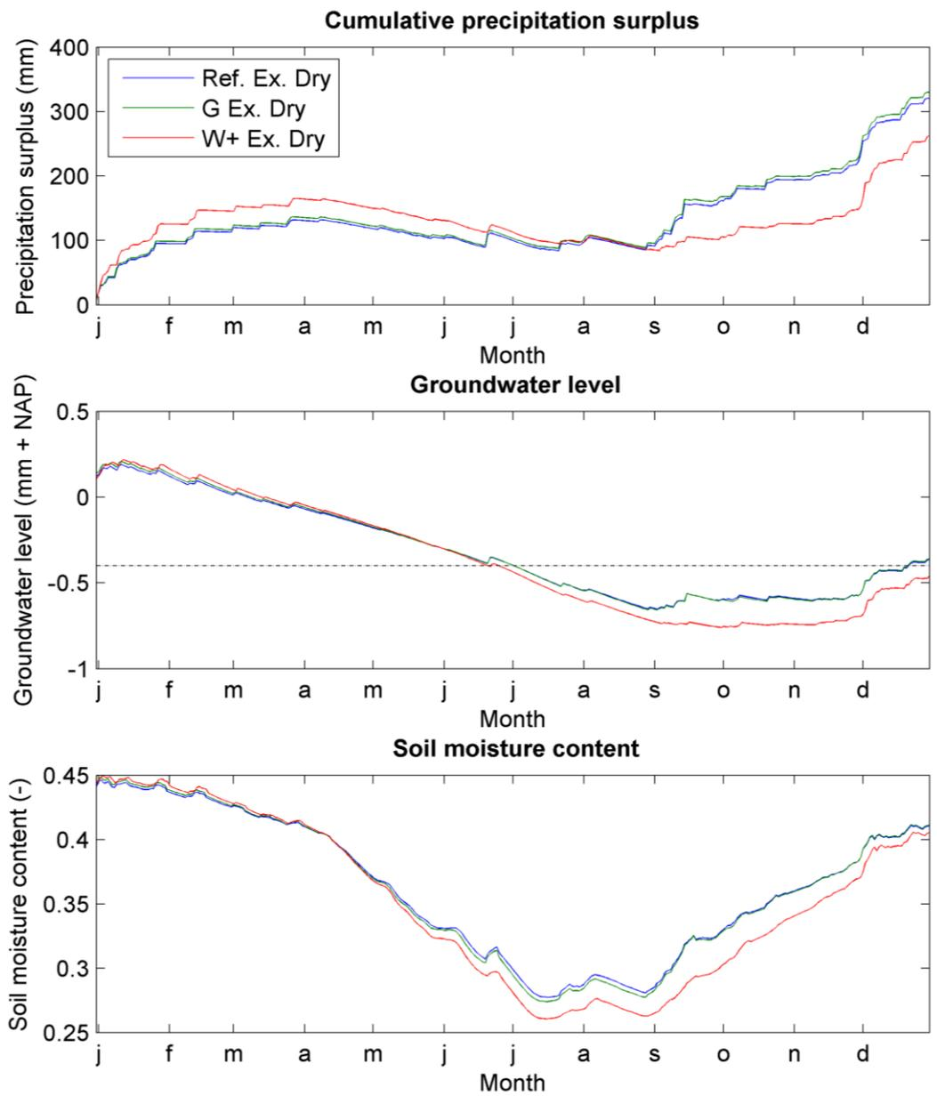
Figure 13.7. The simulated cumulative precipitation surplus (precipitation - evaporation), groundwater levels and soil moisture content over the 'Extremely dry' years of the 'Reference' (blue line), 'G' (green) and 'W+' (red) climate scenarios for the Prinseneiland. The dotted line in the middle graph indicates the surface water level.
