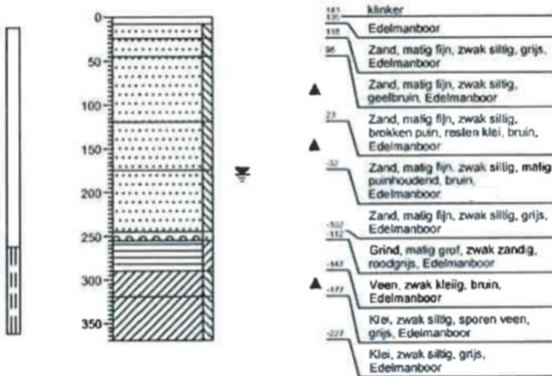
Figure 14.3. Soil survey on the location of piezometer C05269
