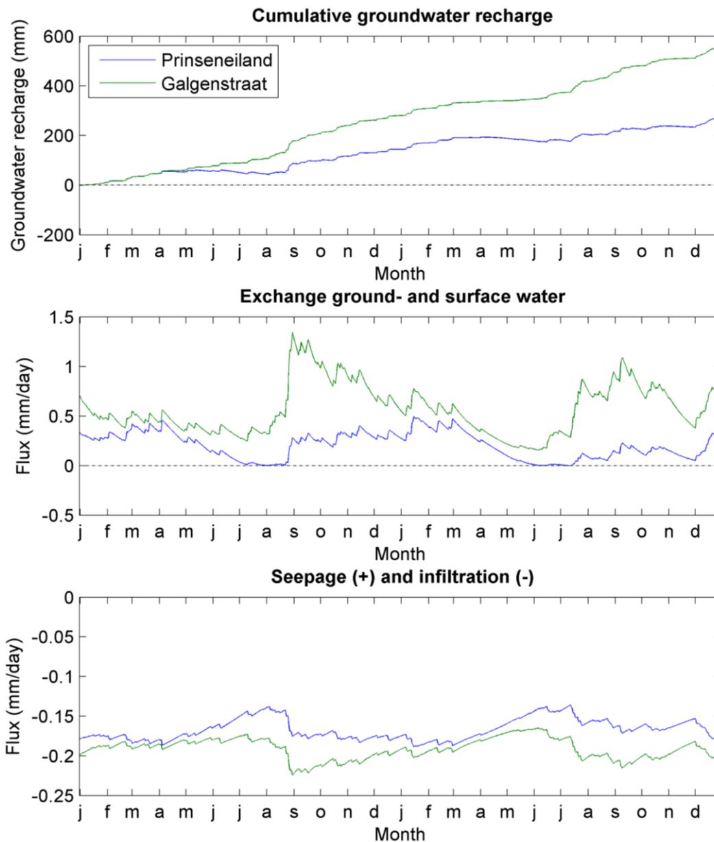
Figure 6.4. The simulated groundwater recharge, the flow of water between the urban ground- and the regional surface water and the flow of water between the urban and regional groundwater bodies over the years 2010 and 2011 for the Prinseneiland and the measuring location at the Galgenstraat.
