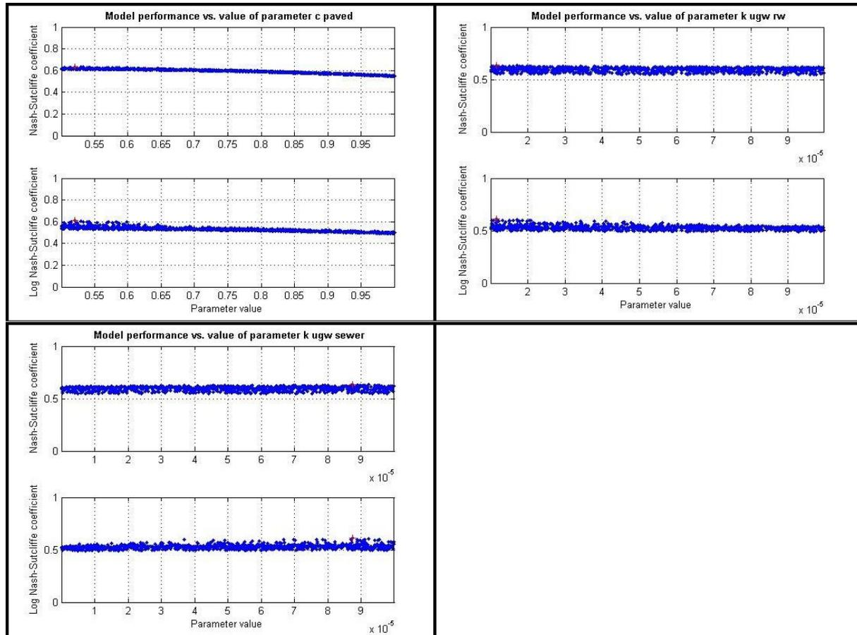
Figure 12.3. Performance of the model as a function of the values of the model parameters. The performance of the model is plotted vs. the values of 'c\_paved' (top left pair), 'k\_ugw\_rw' (top right pair) and 'k\_ugw\_sewer' (bottom left). Each blue dot corresponds with the results of one Monte-Carlo run. The red cross indicates the calculated optimal parameter value.
