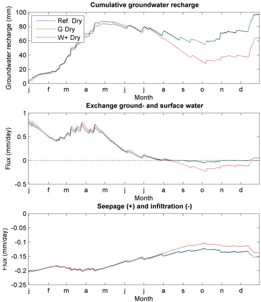
Figure 13.5. The simulated groundwater recharge, the flow of water between the urban ground- and the regional surface water and the flow between the urban and regional groundwater bodies over the 'Dry' years of the 'Reference' (blue line), 'G' (green) and 'W+' (red) climate scenarios for the Prinseneiland.
