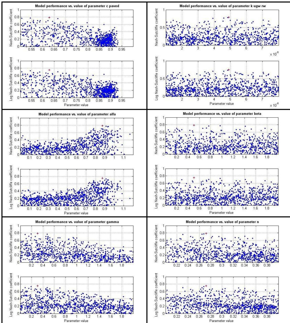
Figure 12.2. Performance of the model as a function of the values of the model parameters. The performance of the model is plotted vs. the values of 'c\_paved' (top left pair), 'k\_ugw\_rw' (top right pair), 'alfa' (middle left), 'beta' (middle right), 'gamma' (bottom left) and 'n' (bottom right). Each blue dot corresponds with the results of one Monte-Carlo run. The red cross indicates the calculated optimal parameter value.
