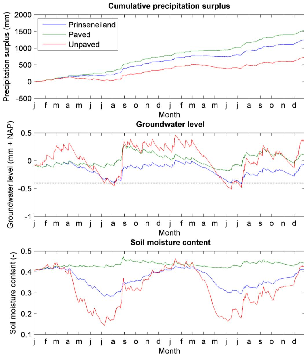
Figure 6.5. The simulated cumulative precipitation surplus (precipitation - evaporation), groundwater levels and soil moisture content over the years 2010 and 2011 for the Prinseneiland (blue line) and a completely paved (green) and unpaved Prinseneiland (red). The dotted line in the middle graph indicates the surface water level.
