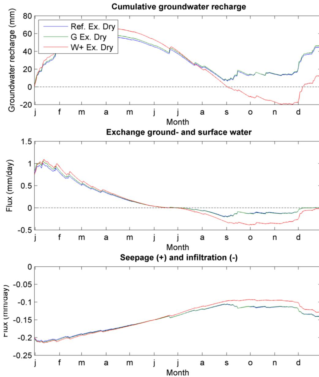
Figure 13.8. The simulated groundwater recharge, the flow of water between the urban ground- and the regional surface water and the flow between the urban and regional groundwater bodies over the 'Extremely dry' years of the 'Reference' (blue line), 'G' (green) and 'W+' (red) climate scenarios for the Prinseneiland.
