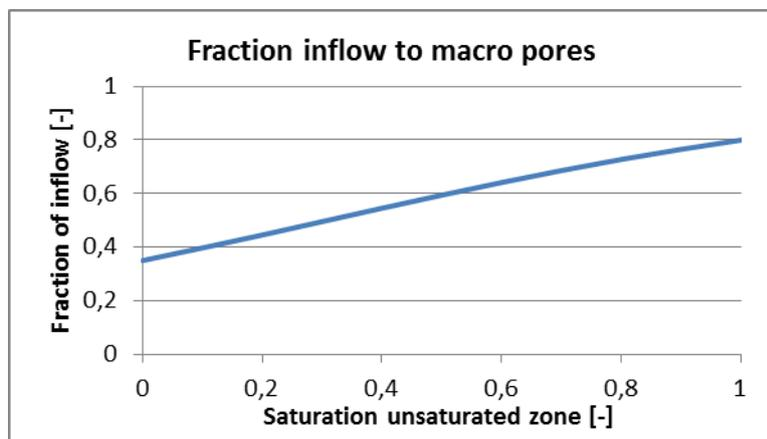
Figure 5.3. Fraction of the inflow into the unsaturated zone that is routed to through the macro pores as a function of the saturation of the unsaturated zone bucket.
