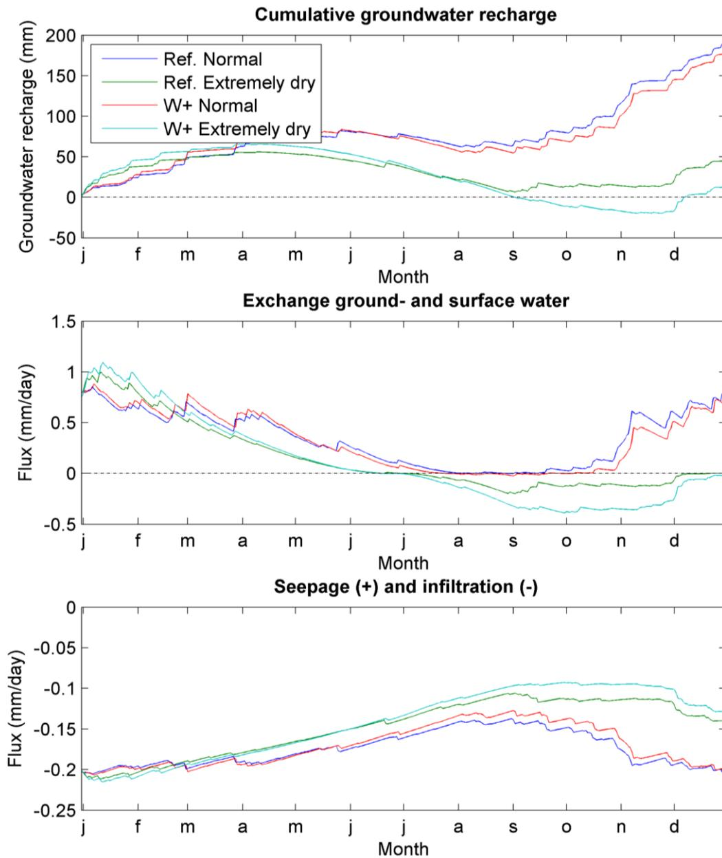
Figure 6.13. The simulated groundwater recharge, the flow of water between the urban ground- and the regional surface water and the flow between the urban and regional groundwater bodies over the scenario years 'Reference, Normal' (blue line), 'Reference, Extremely dry' (green), 'W+, Normal' (red) and 'W+, Extremely Dry' (cyan) for the Prinseneiland.
