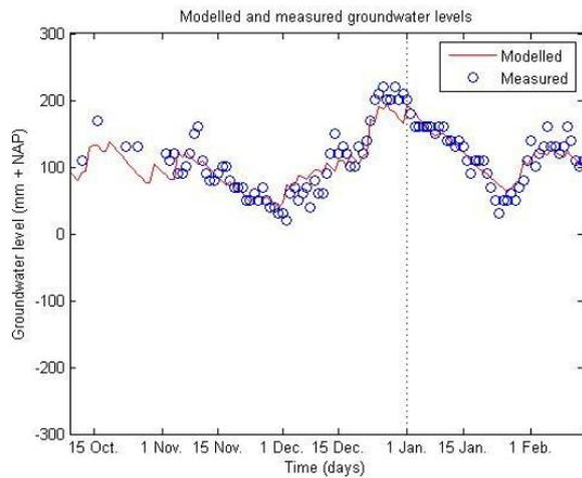
Figure 5.6. Simulated groundwater levels at the Galgenstraat with the optimal parameter values according to both performance indicators from Oct. 2012-Feb. 2013.
