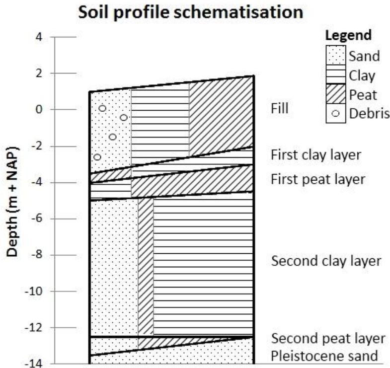
Figure 3.5. Schematisation of the soil profile of the Prinseneiland. The lines between the soil layers indicate differences in depth of the layer boundaries over the island. The shown ratios of soil material in a layer give a crude indication of the extent to which the material is generally present over the area. Even over short distances between locations the ratios can differ significantly from each other and the ratios in this figure.
