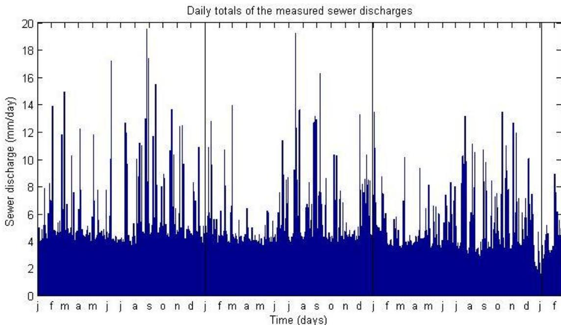
Figure 4.3. The daily totals of the measured sewer discharges of the Prinseneiland over the period Jan. 2010 - Feb. 2013. The labels on the x-axis indicate the first day of the month.
