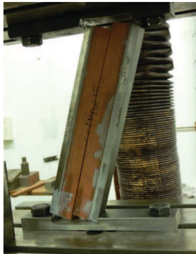
Figure 11: Massaranduba specimen: Failure of 0% in the glueline.
