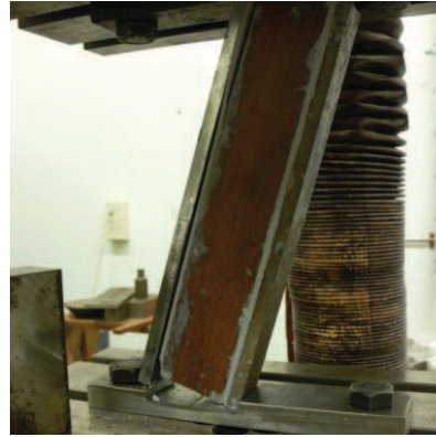
Figure 10: Massaranduba specimen: Failure of 100% in the glueline.
