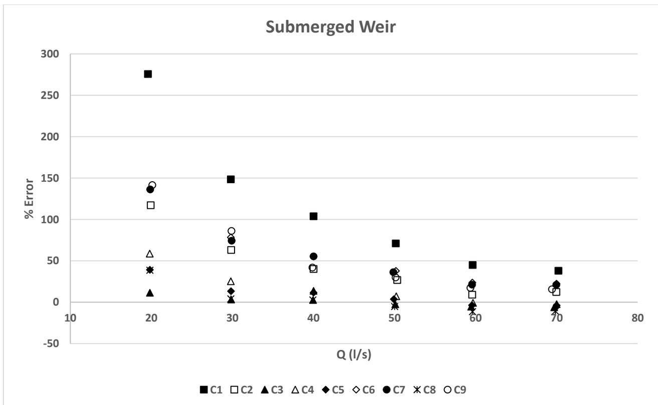
Figure 3. Comparison of measured and modeled (Eqns. 2 and 3) discharges at submerged weir cases.
