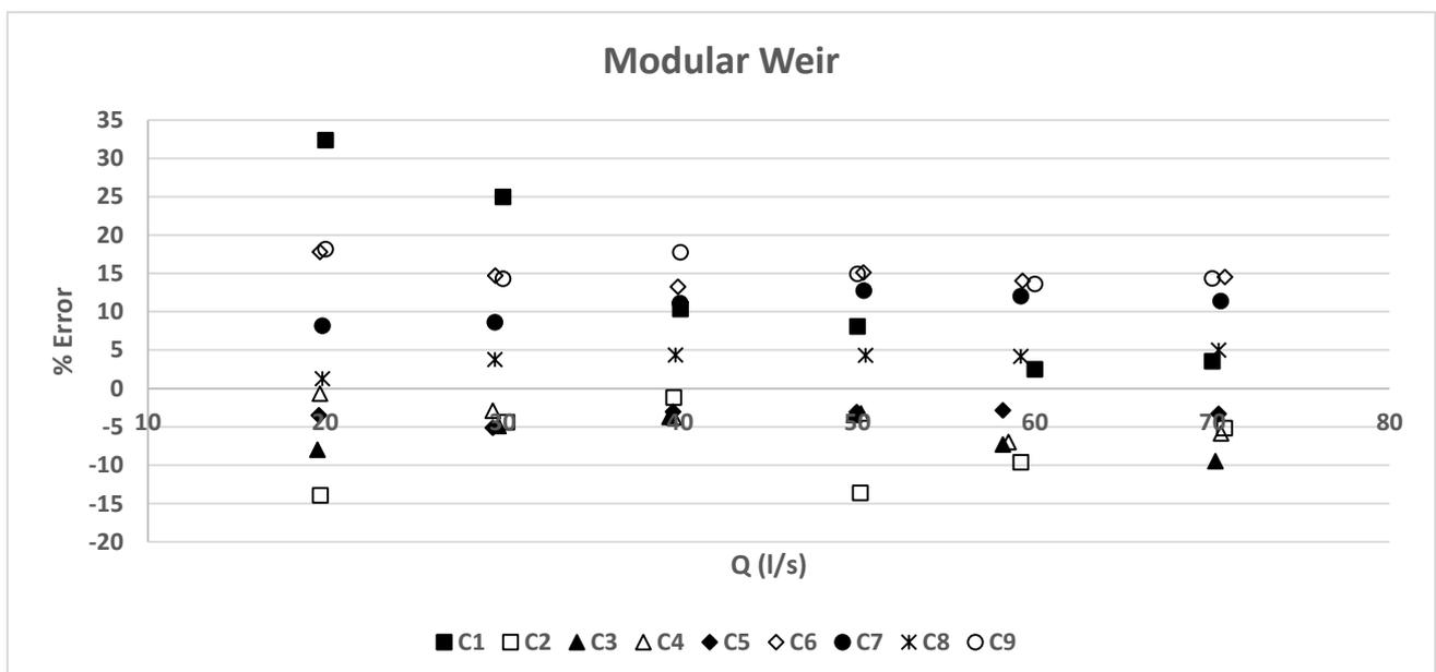
**Figure 2.** Comparison of measured and modeled (Eqn. 1) discharges at modular weir cases.
