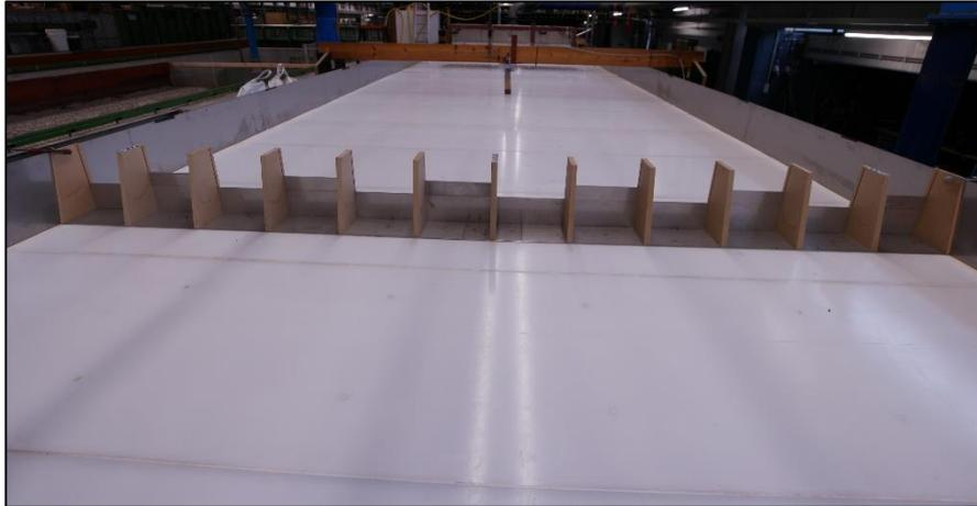
**Figure 1.** Flume view from the downstream of the weir structure (Weir configuration in figure is C4)
