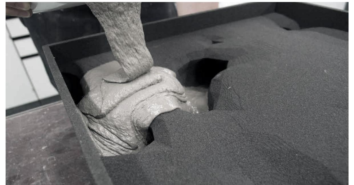
Figure 2.46. Casting of UHPFRC into the binder jet 3D printed formwork, ETH Zurich (Jipa et al., 2016).
