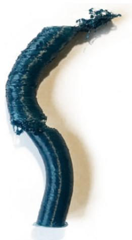
Figure 6.19. Problems in extrusion printing due to shifting of layer by vibrating bed
