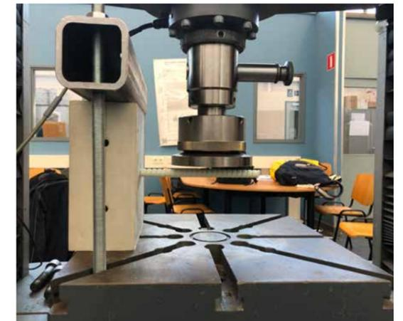
Figure 6.12b. Laboratory setup of the concrete mass with 2 x 10 mm diameter tubes and the reinforcement dowel with 33 mm concrete cover from both of their edges. (Author)
