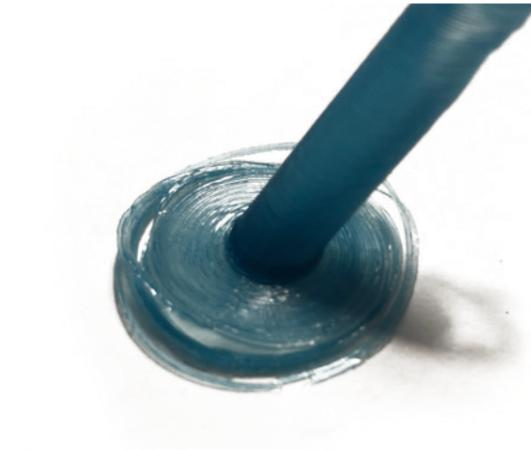
Figure 6.23. Problems in extrusion printing due to improper adhesion to bed
