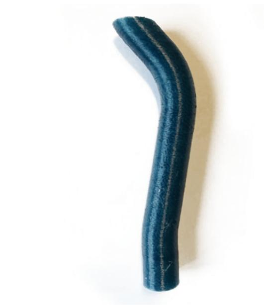
Figure 6.25. A good quality of extrusion printing
