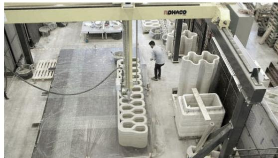
Figure 2.47. Test 3D printing of a segment for a bridge, Project Milestone by TU/e (Mlot, 2018).
