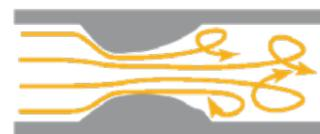
Figure 7.1a. Turbulent flow
