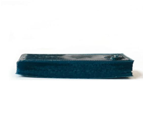
Figure 6.22. Problems in extrusion printing due to geometry warping
