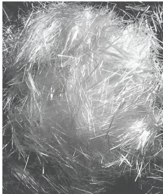
Figure 2.23. Glass fibres for concrete mixture (alibaba.com)
