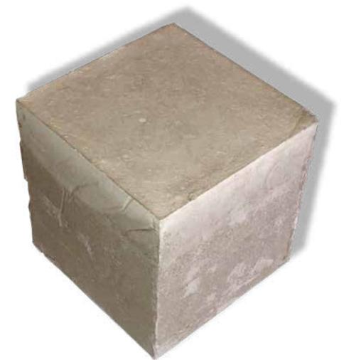
Figure 6.1a. Weber Beamix with fibres by Saint Gobain, concrete cube of 100 x 100 x 100 mm. (Author)
