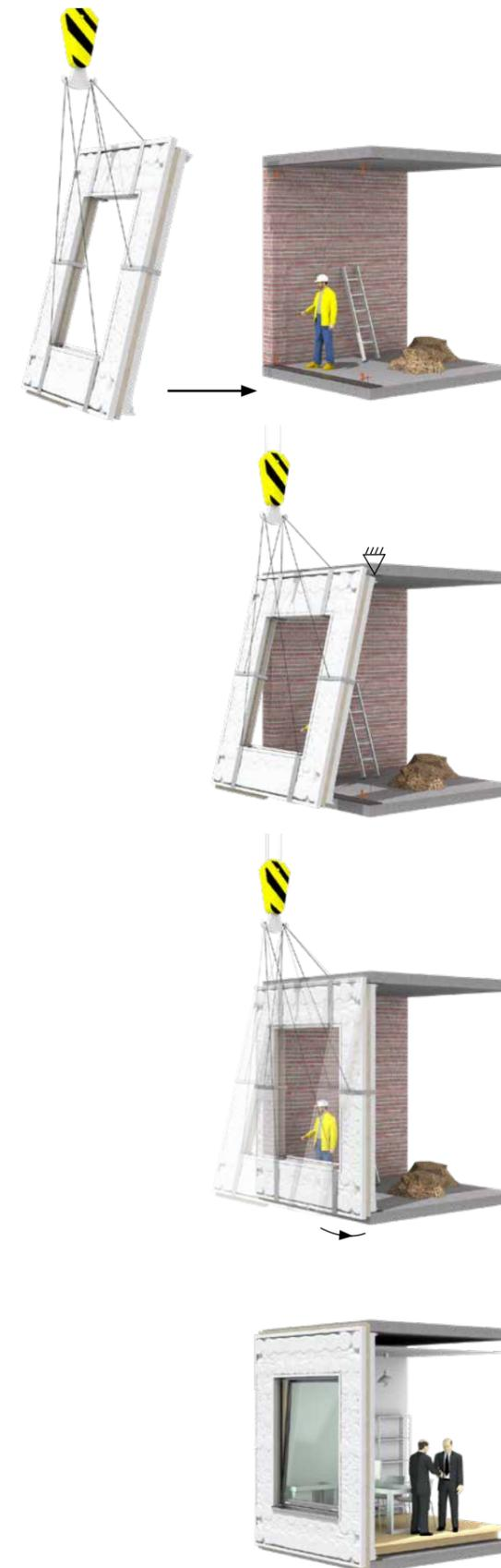
The façade panel is pre-fabricated and transported to the built site. It is lifted to position by a crane using 3-point tilt-up system.
