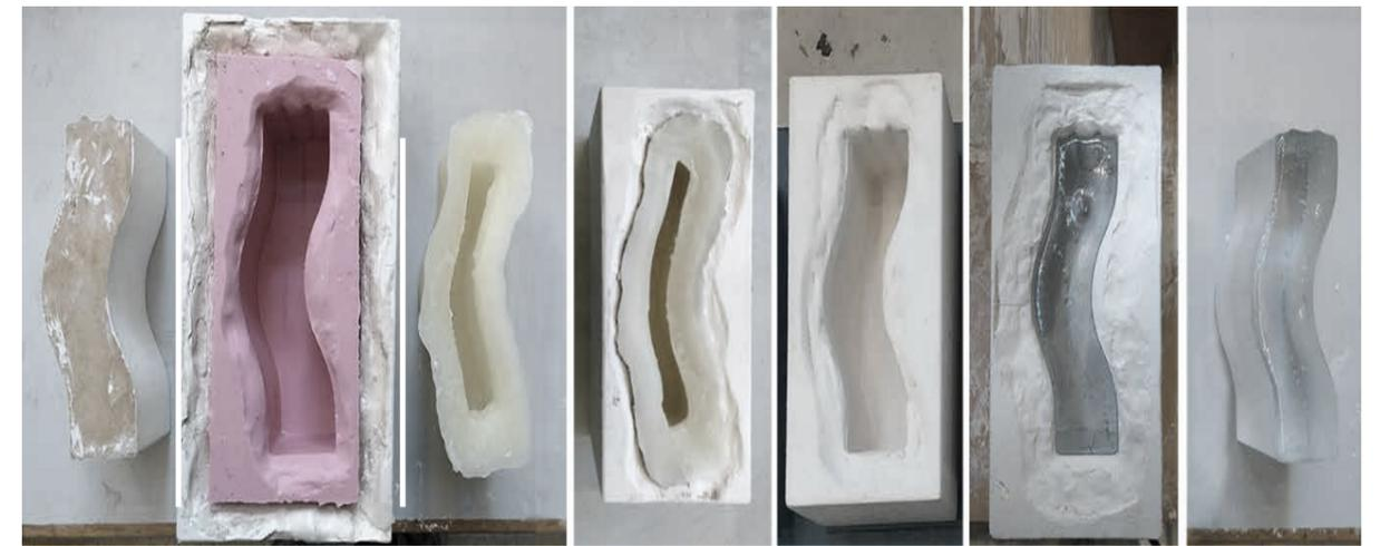
Figure 2.53. Production steps from MDF mould to final glass model (Bristogianni, Oikonomopoulou, Veer, Snijder, & Nijse, 2017).
