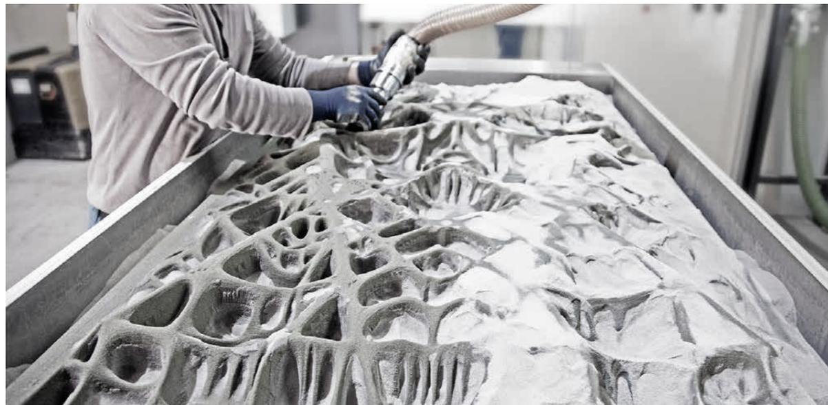
Figure 2.52. Post processing of the fabricated concrete slab by binder jetting by ETH Zurich (Jipa et al., 2016).
