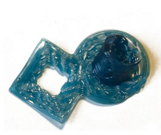
Figure 6.18. Problems in extrusion printing due to lumping of material
