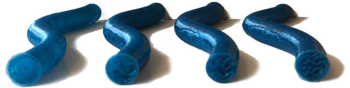
Figure 6.16. Infill geometry used for printing tubes with varying percentage for loading test. (Author)
