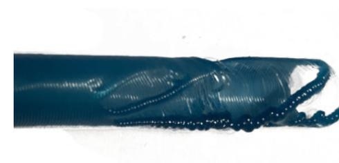
Figure 6.20. Problems in extrusion printing slow cooling of layers
