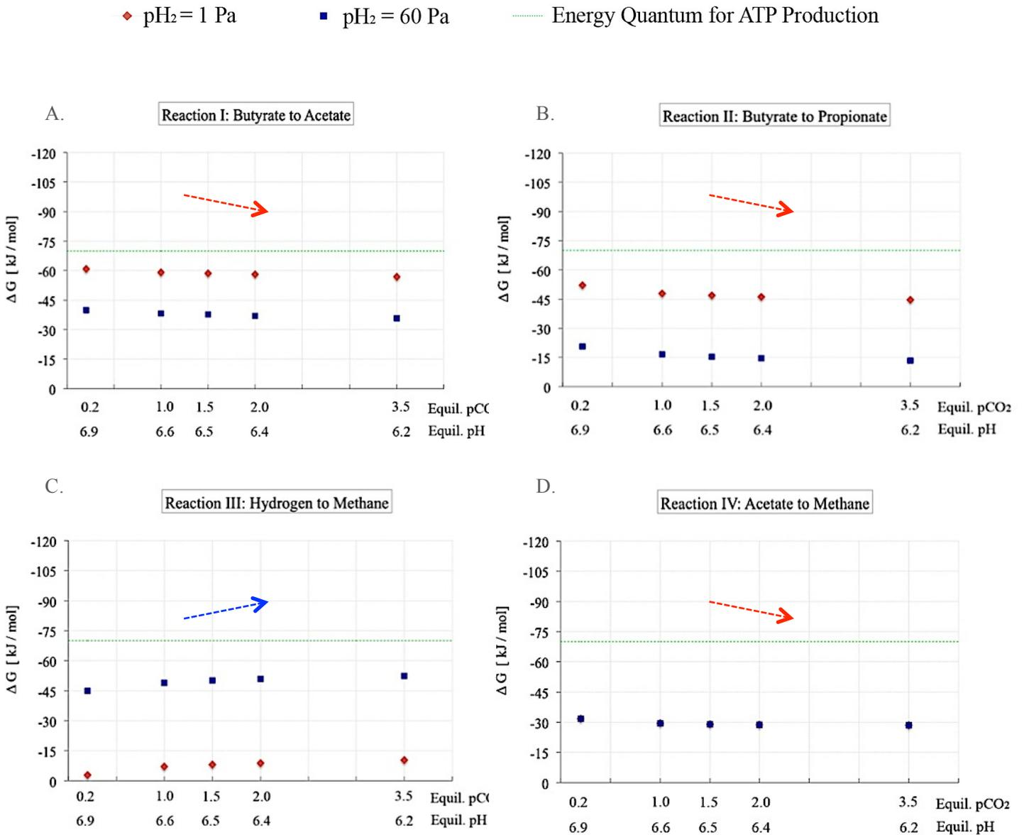
Figure 4-8. Effect of increasing  $\text{pCO}_2$ 's on the energy yields for the main catabolic reactions in butyrate fermentation: (A). Reaction I: Butyrate to Acetate; (B). Reaction II: Butyrate to Propionate; (C). Reaction III: Hydrogen to Methane; (D). Reaction IV: Acetate to Methane.
