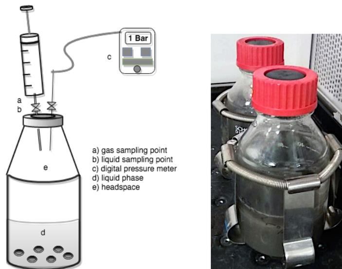
Figure 3-1. Schematic representation of the experimental set-up for batch experiments conducted at 0.2 and 1 bar pCO<sub>2</sub>
