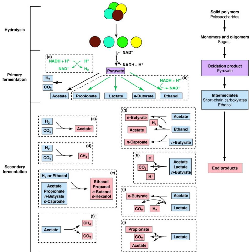
Figure 2-2. Pyruvate as a central metabolite in the fermentation of solid polymers by undefined mixed cultures (Source: Agler et al., 2011)
