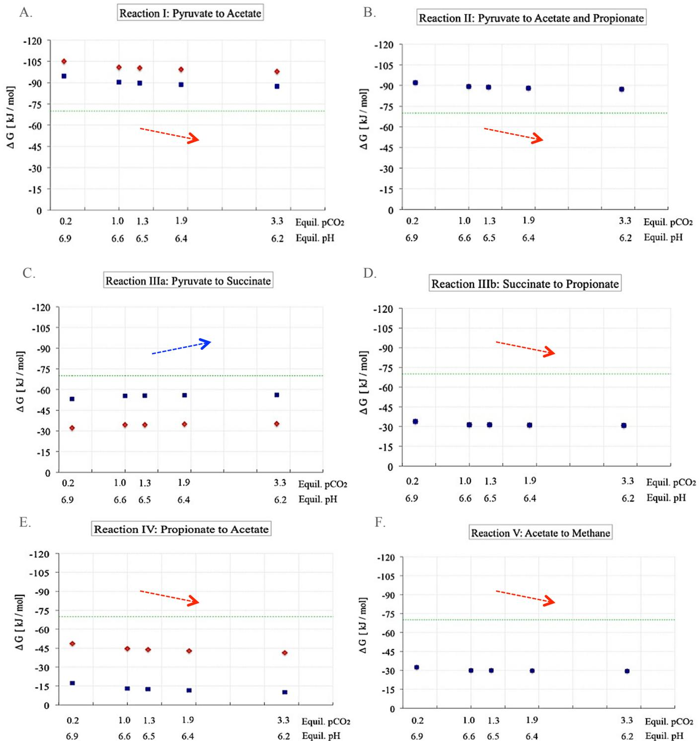
Figure 4-7. Effect of increasing pCO<sub>2</sub>'s on the energy yields for the main catabolic reactions in pyruvate fermentation: (A). Reaction I: Pyruvate to Acetate; (B). Reaction II: Pyruvate to Acetate and Propionate; (C). Reaction IIIa: Pyruvate to Succinate; (D). Reaction IIIb: Succinate to Propionate; (E). Reaction IV: Propionate to Acetate; (F). Reaction V: Acetate to Methane.
