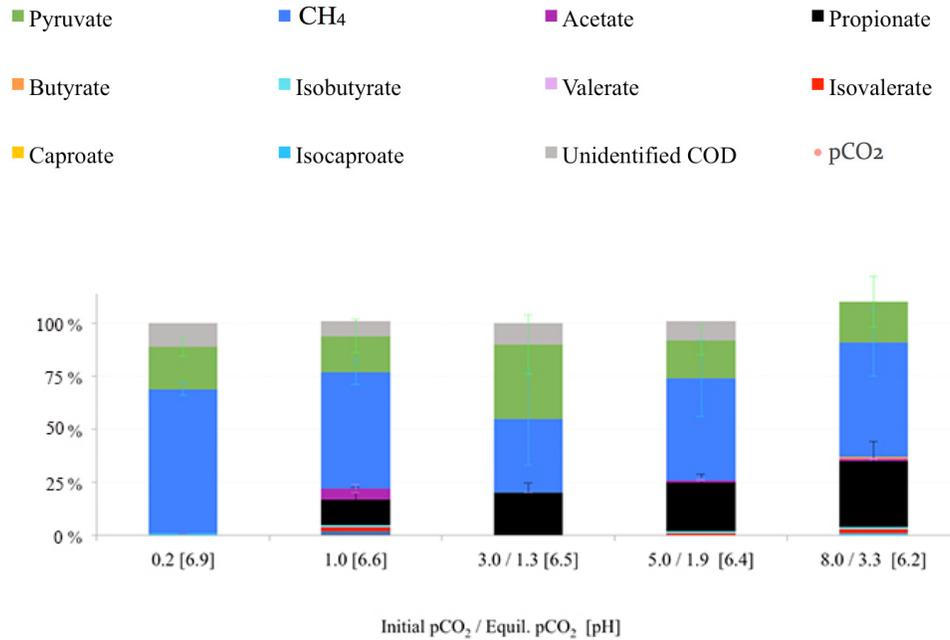
Figure 4-2. Overview of the product spectrums at 5 different CO<sub>2</sub> partial pressures at the end of the pyruvate experiments
