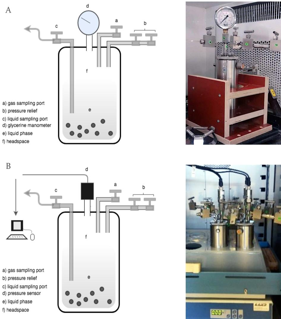
Figure 3-2. Schematic representation of the experimental set-up for batch experiments conducted at 3.0, 5.0 and 8.0 bar  $p\text{CO}_2$ . (A) Reactors fitted with glycerin manometers. (B) Reactors fitted with pressure sensors.
