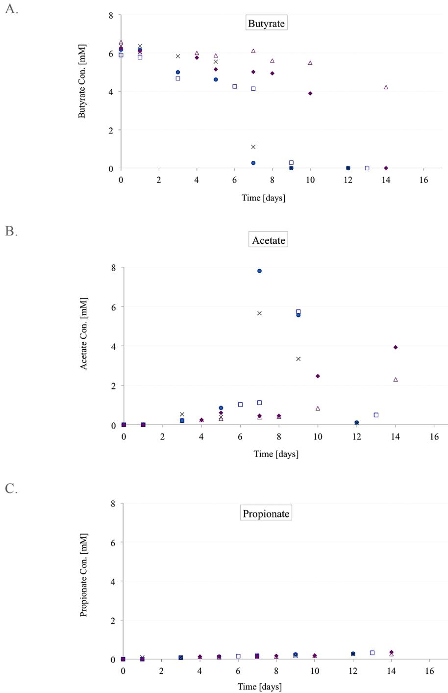
Figure 4-10. Changes in the concentration of the main metabolites in the butyrate experiments over time: (A). Butyrate, (B). Acetate and (C). Propionate
