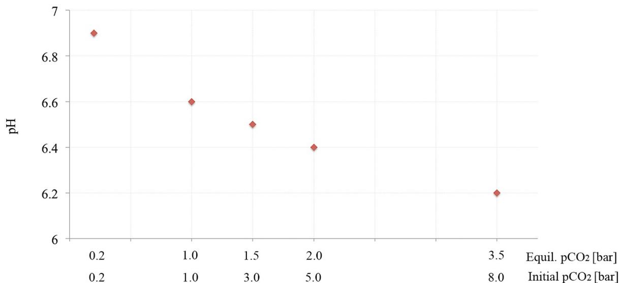
Figure 3-3. Changes in the liquid broth's pH in response to the operating/equilibrium CO<sub>2</sub> partial pressures
