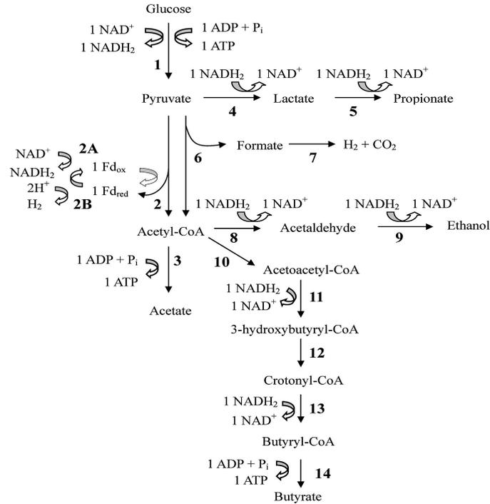
Figure 2-3. Metabolic pathways of mixed-acid fermentation of glucose. (*Prescott et al., 2002*)
