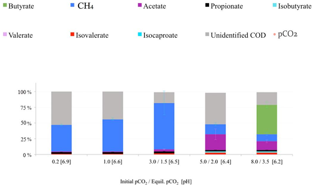
Figure 4-5. Overview of the product spectrums at 5 different CO<sub>2</sub> partial pressures at the end of the butyrate experiments
