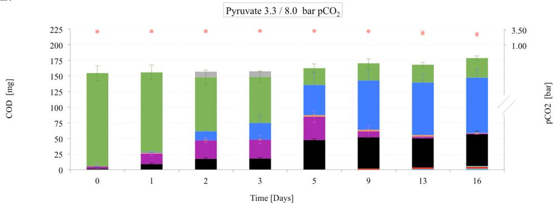
Figure 4-1. Product spectrum in the fermentative degradation of pyruvate at 5 different CO<sub>2</sub> partial pressures: (A). 0.2 bar; (B). 1.0 bar; (C). 3.0 bar; (D). 5.0 bar; (E). 8.0 bar
