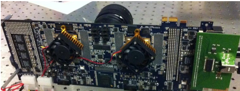
Figure 2.13. Physical appearance of the camera based on SwissSPAD; a daughterboard hosting the chip is electrically connected to a motherboard hosting two Xilinx-IV that process the raw frames generated by the chip and format them to send them through a USB2 link.
