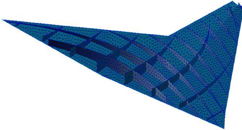
Figure 2.5: Typical SpaRibs design in a wing structure. Adapted from [57]
