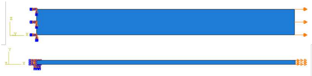
Figure 3.2: Load case for tension test
