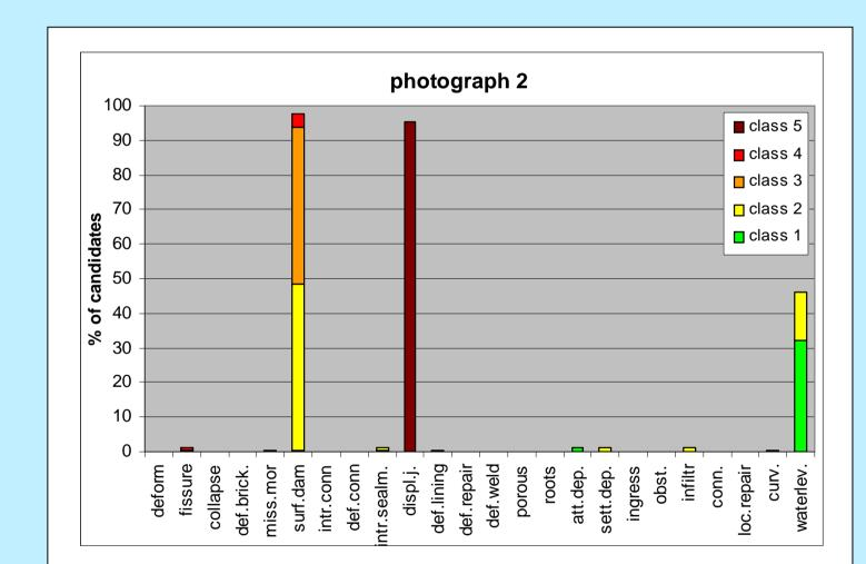
From the graph it is clear that the defects of the sewer shown in this photograph were easy to recognize: surface damage and a displaced joint (it is not obligatory to denote water level class 1: h< 10% of the diameter).
