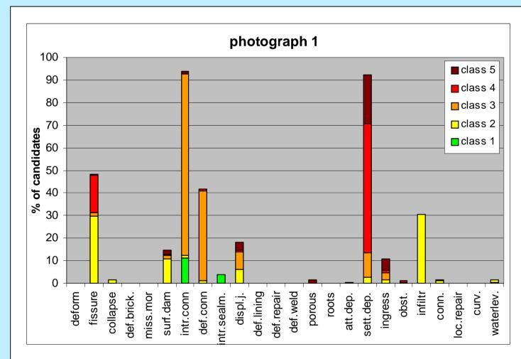
The responses of the candidates do not make clear what kind of defects were present in the photographed sewer. For this sewer the candidates did not agree on the presence of the defects fissure, defective connection, displaced joint and infiltration.
