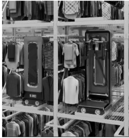
ASRS (Automated Storage and Retrieval Systems) for garments on hangers - first patent developed by the US firm Planiform in 2022.
