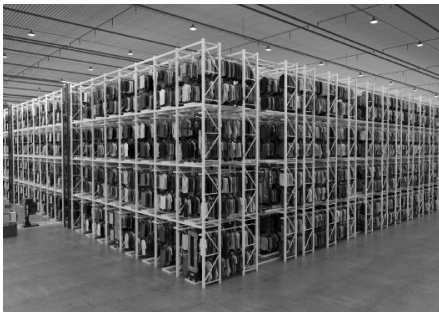
ASRS (Automated Storage and Retrieval Systems) for garments on hangers - first patent developed by the US firm Planiform in 2022.
