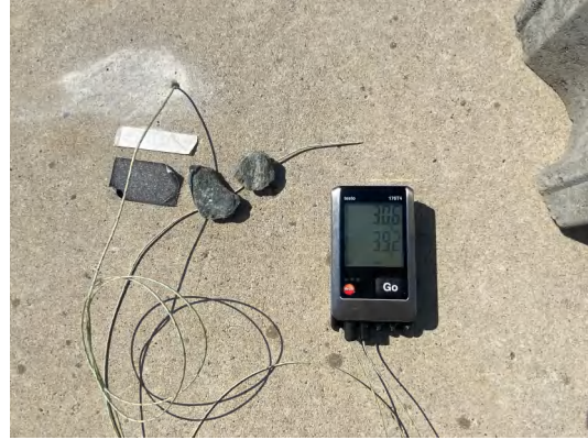
Figure 4: Testo 176T4 for Surface and Bottom Temperature of Concrete
