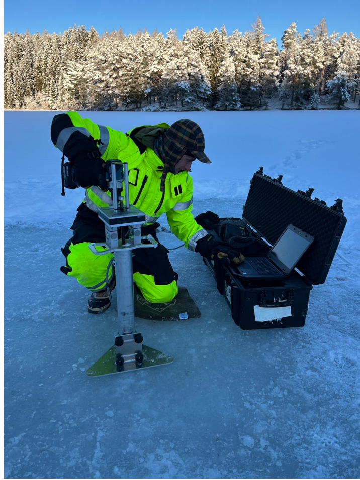
Figure 3.5: Photograph of the BHJ including field laptop, transportation case and logger box in field testing mode.
