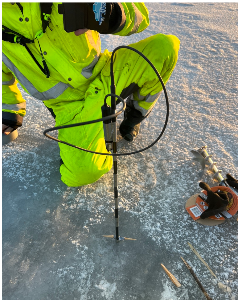
Figure 3.8: Photograph of the thermistor string installed at Hjellobtn to monitor the vertical temperature profile.
