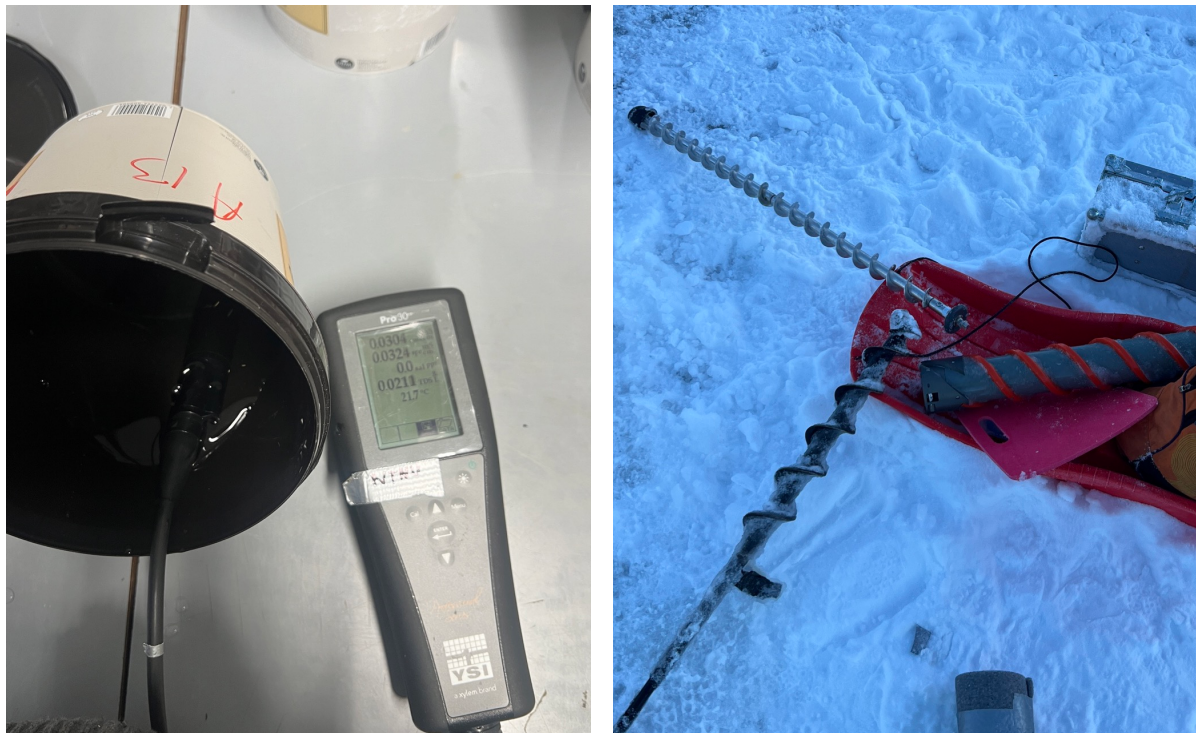
(a) The Salinity measurement setup at the NTNU using melted ice core segments. Measurements were carried out using the YSI Pro 30 conductivity meter.
