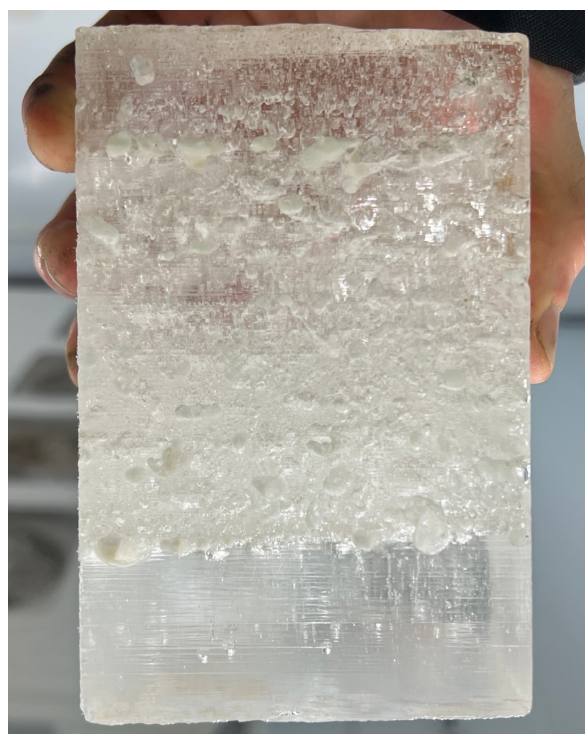
(b) Sawed block of Hjellbotn ice in the cold lab at NTNU. Retrieved for density measurements.
