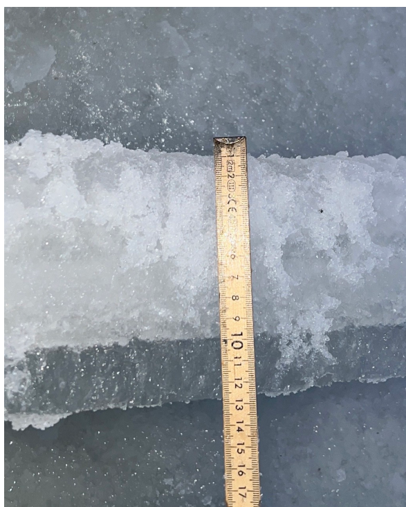
(a) Block of ice after retrieval at Hjellbotn test site, measuring approximately 13 cm in thickness.
