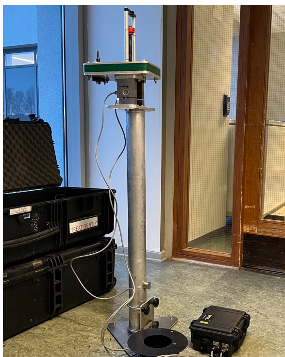
(a) Photograph of the Borehole Jack used for in-situ sea ice strength testing. The steel cylinder houses a horizontally oriented piston that can be extended to apply a force against the ice borehole wall. Photo taken at the NTNU, Trondheim.
