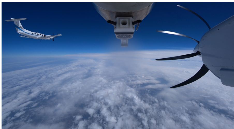
Figure 2. A picture taken from the Egrett's left landing gear camera, with the propeller of the Egrett (on the right) and the CAPS probe (on the top), shortly before going into formation flight with the Piper Cheyenne (400LS, registration 30 N92EV). The emission aircraft equipped with a two-engine turboprop of type Garrett/Honeywell TPE 331-14 was chased at altitudes between 7.6 and 10.4 km.
