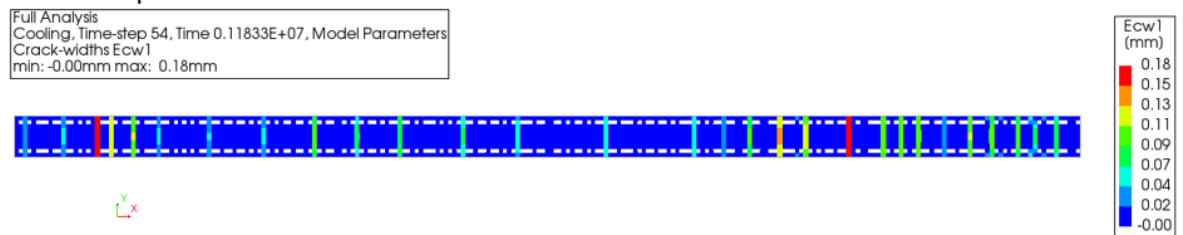
Figure B.8: Resulting crack pattern when the final temperature is higher than the initial temperature
