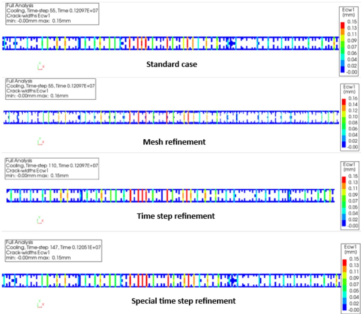
Figure C.5: Comparison of the crack width results of the mesh refinement, time-step dependency analysis, the special time-step analysis and the standard model
