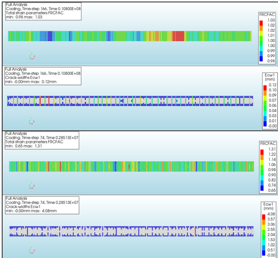
Figure 4.12: Example results, a similar random field with a different standard deviation ( \sigma ) displays two types of behaviour. Multiple distributed smaller cracks (upper panel, \sigma = 1\% ) or a single localized large crack (lower panel, \sigma = 15\% )
