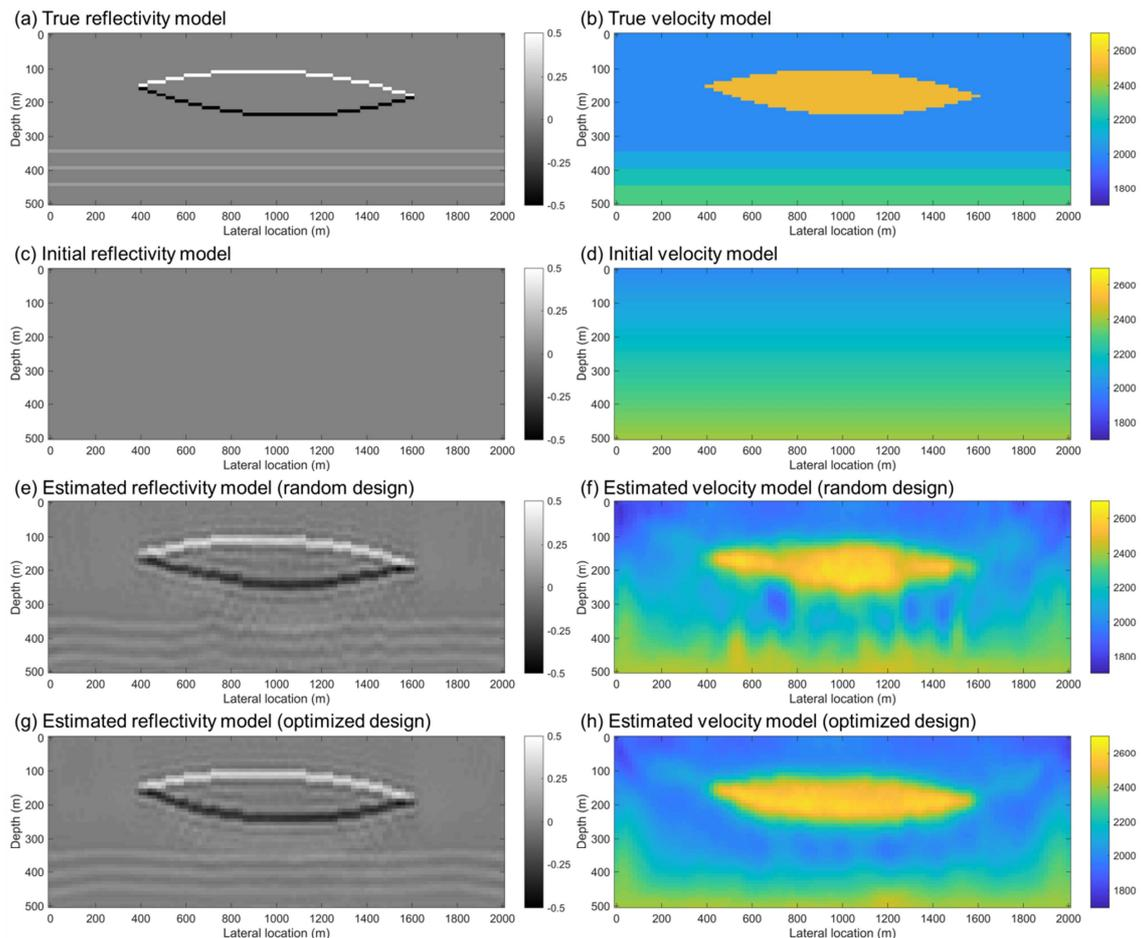
**Figure 4** Comparison of JMI results between two different design schemes. The notable enhancement in the performance of JMI due solely to the choice of survey parameters is easily recognizable.
