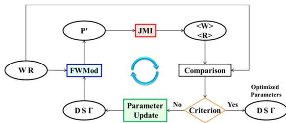
**Figure 1** The overall iterative survey-design workflow. FMWod in the blue box generates blended and irregularly sampled data ( $\mathbf{P}'$ ). JMI in the red box estimates reflectivity and velocity models using a given design. GA and CNN embedded into the green box update the survey parameters.
