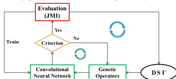
**Figure 2** The scheme focusing on the procedure to optimize  $\mathbf{D}$ ,  $\mathbf{S}$  and  $\mathbf{\Gamma}$ . The GA repeatedly produces these operates till the criterion in the CNN is met. They are subsequently fed into JMI to obtain estimates of reflectivity and velocity. The CNN is trained at each iteration using actual JMI results.
