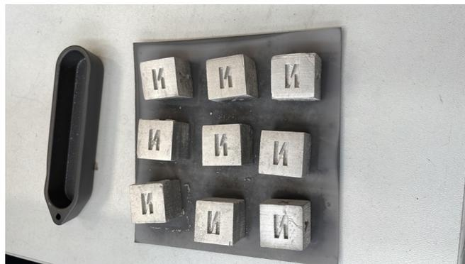
(a) Sintered Samples (with N-face up)
