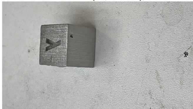
(b) Sintered samples with slight surface damage
