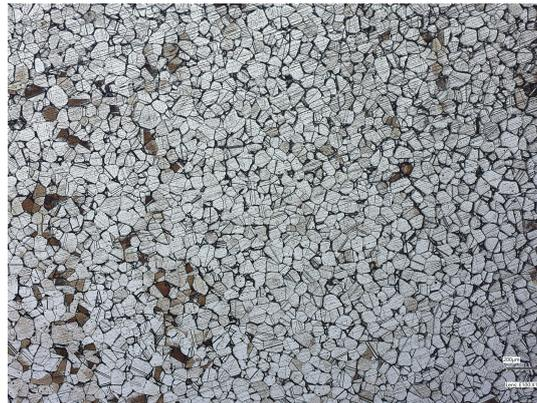
(c) Particle size  $<25\ \mu\text{m}$ , sintered in Vacuum
