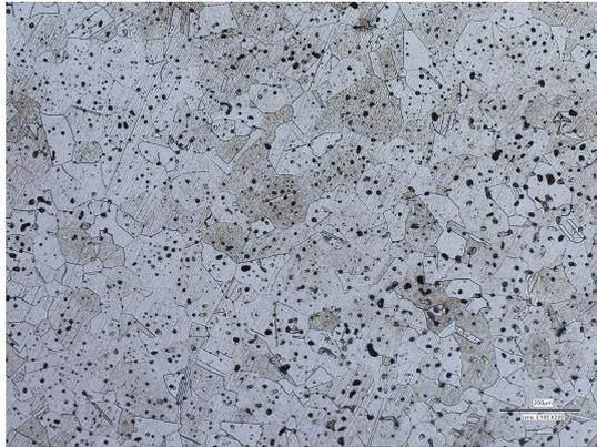
(a) Particle size  $<18\ \mu\text{m}$ , sintered in Ar
