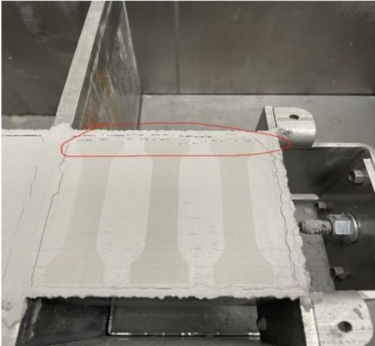
(b) Edge cracks make dog-bone fracture
