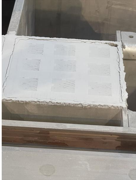
**Figure 4.3:** Powder leakage at the edge of printing platform during printing process
