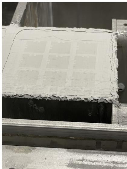
Figure 4.7: Powder leakage and cracks during the printing
