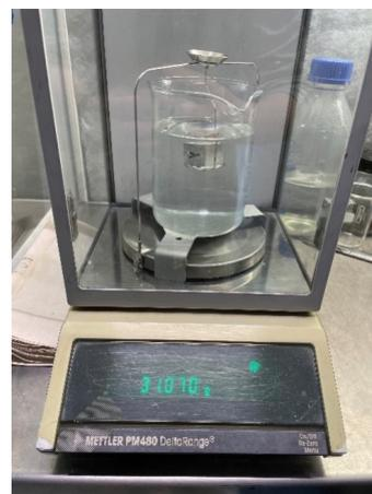
(b) Archimede's method for density measurement
