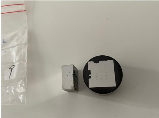
(a) Polished samples for hardness test
