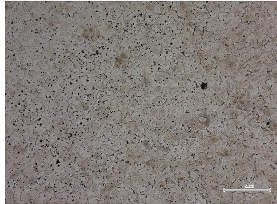
(b) Particle size  $<25\ \mu\text{m}$ , sintered in Ar
