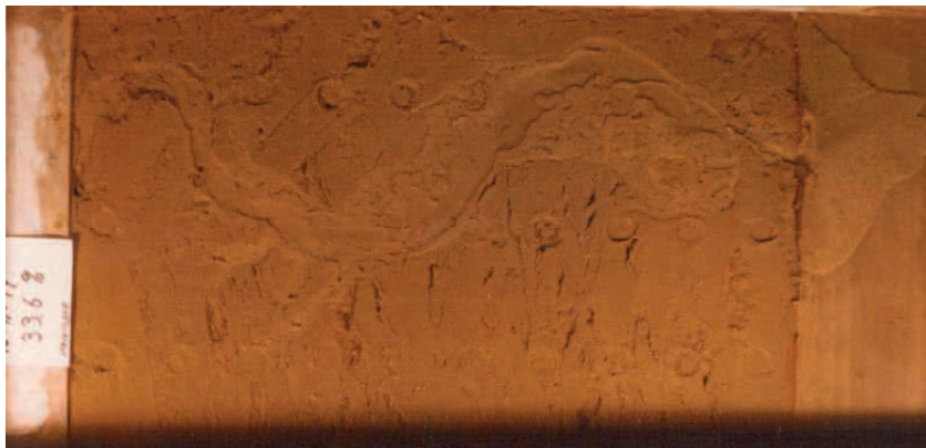
Figure 2 Pipe development and crater formation visible after removal of the clay layer
