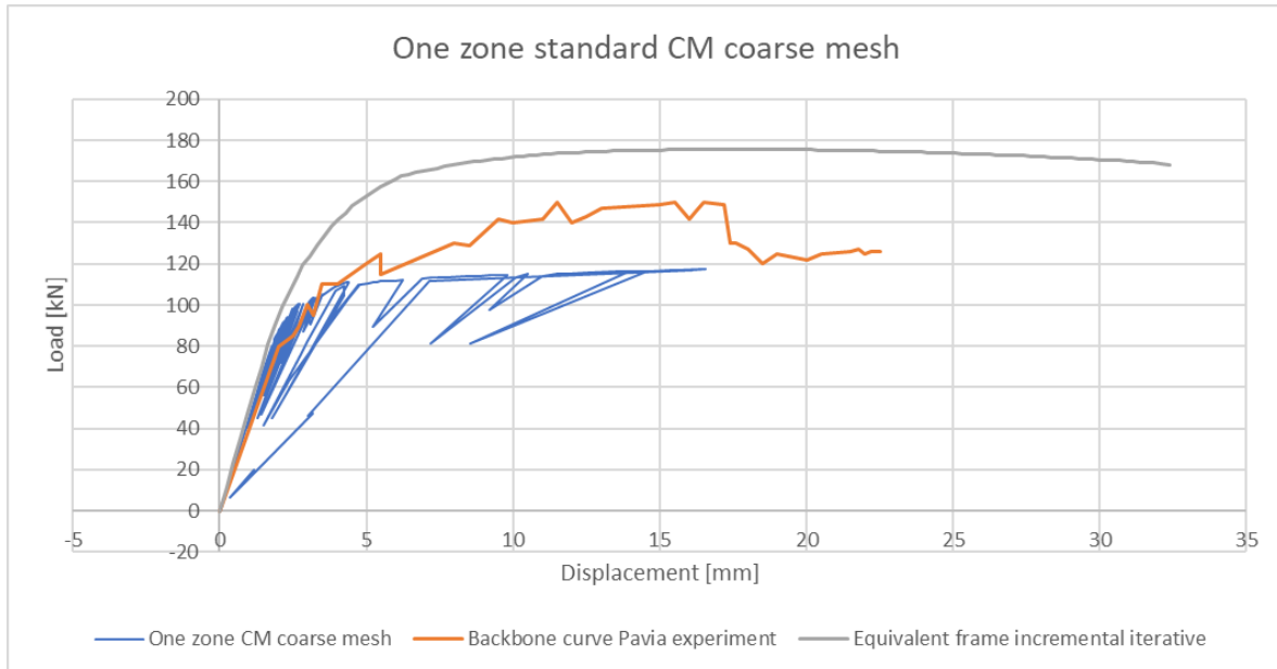
Figure 4.53; Load-displacement curve; CM coarse mesh
