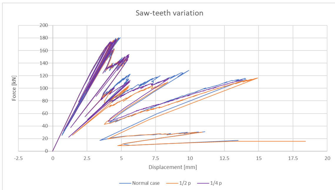
Figure 5.37; Variation in the number of saw-teeth for the three-zoned beam model
