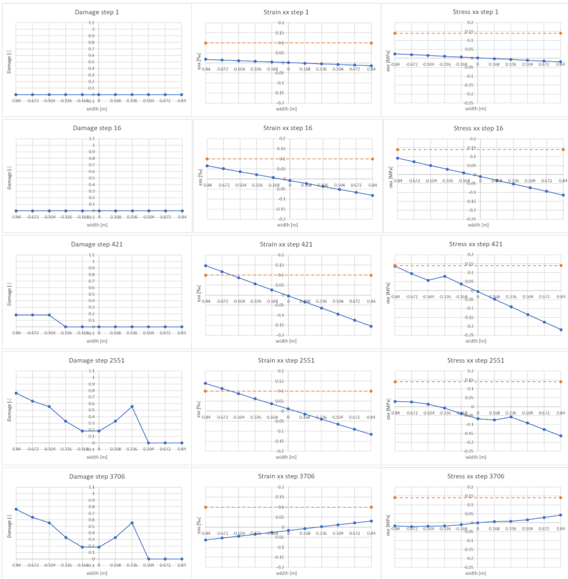
Figure 5.15; Damage, strain \epsilon_{xx} and stress \sigma_{xx} in element 208, analysis steps: 1, 16, 421, 2551 and 3706
