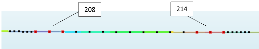
Figure 5.12; Element 208 and 214 in the right spandrel of the first floor
