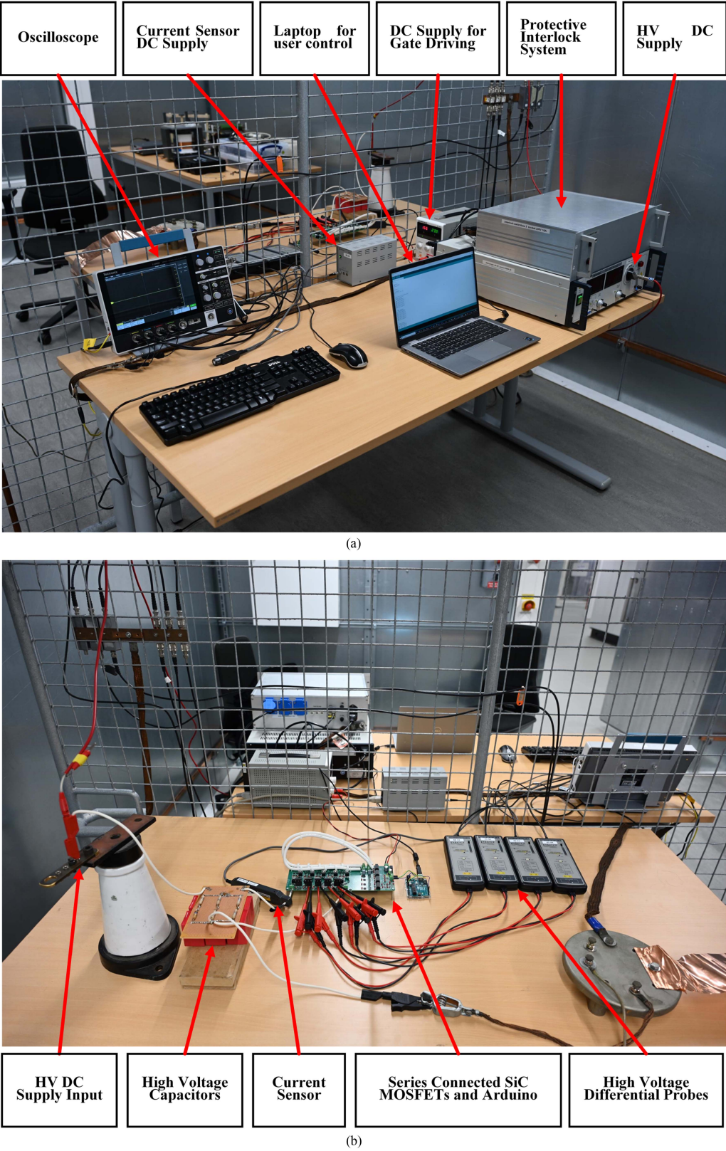
FIGURE 26. (a) Control and monitoring setup installed outside the Faraday's cage with 24-V dc supply, Heinzinger HVdc supply, oscilloscope, and a PC to input user-defined signal to Arduino. (b) High-voltage test setup inside protective Faraday's cage with high-voltage capacitors, current sensor, series-connected MOSFETs prototype printed circuit board (PCB), Arduino, and four high-voltage active differential probes attached to the source-drain terminals of four series-connected SiC MOSFETs.
