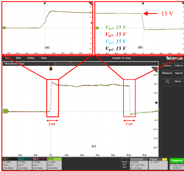
FIGURE 27. Gate-to-source ( V_{gs} ) voltage across four SiC MOSFETs in series during turn-ON and turn-OFF.
