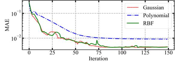
Fig. 4. Evolution of the maximal absolute error during the fILC learning process when using different kernel functions.
