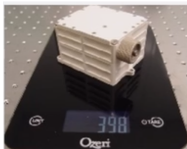
Figure 4.5: The Coherent IS53 diode laser module selected for the power transmission system.
