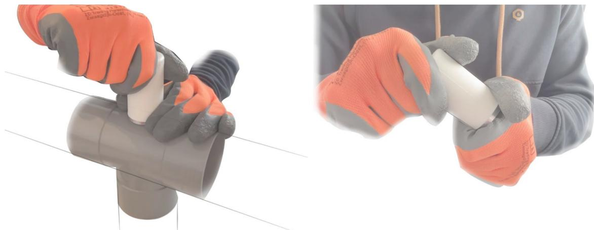
Figure 39: Edge Dynamics sensor node clearance for counter-force (left), clearance for unscrewing in hand (right)
