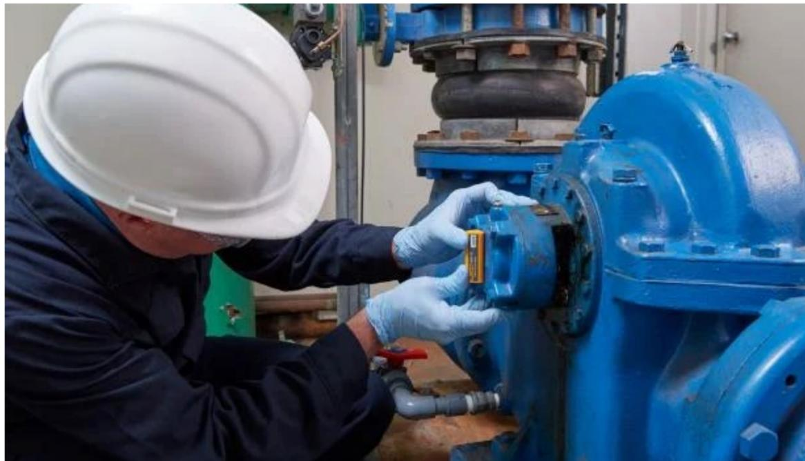
**Figure 18: Mounting Fluke's vibration sensor using epoxy glue (Fluke, n.d.)**
