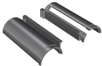
The two structure halves can be injection moulded using a single mould. No undercuts are necessary, resulting in a simple component.
