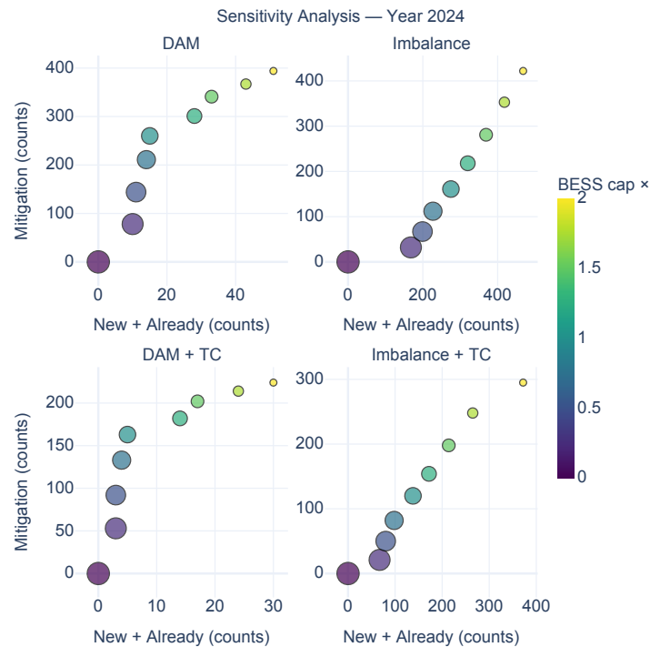
Figure 4.27: Impact of the battery adoption rate scaling on mitigation and new congestion plus charging during already congested events. The bubble size represents the total system costs, with a larger bubble visualizing higher costs.
