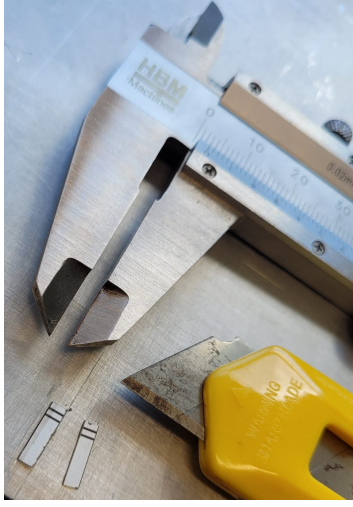
(a) The piezoelectric plates are cut to a length of 10 mm and a width of 2.5 mm using a Stanley knife and a calibrator.
