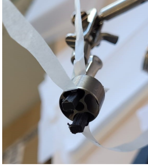
(b) The ring is fixated by a gripper at the inner ring at the back while the piezoelectric plates are glued into place. The black wedges are used to press the plates to the ring.
