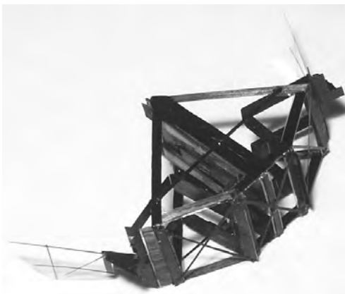
Figure 3.2: The Berkeley MFI, a piezo actuator powered flapping-wing MAV. The MFI is based on two parallel four-bar mechanisms which provide the capability to actively control wing pitching movement. Image from [91]. Copyright: The Biomimetic Millisystems Lab, UC Berkeley, United States, reprinted with permission.
