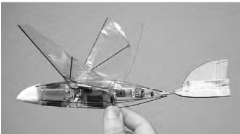
Figure 3.5: The Caltech Microbat [74], a flapping-wing MAV capable of free flight driven by a DC-motor. Image by M. T. Keennon from [74]. Copyright: M. T. Keennon, AeroVironment Inc, Monrovia, CA, United States, reprinted with permission.
