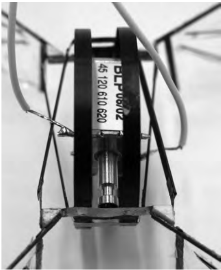
Figure 5.25: The center of Concept 2 ready for testing, including actuator, power leads and wings.
