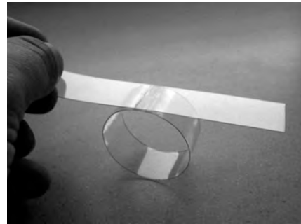
Figure 4.6: Simple compliant extension of the ring to include wings, the wings are deformable part of the structure.
