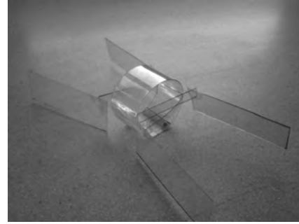
Figure 4.8: Extension of the two winged concept allowing for a more favorable horizontal flapping plane.
