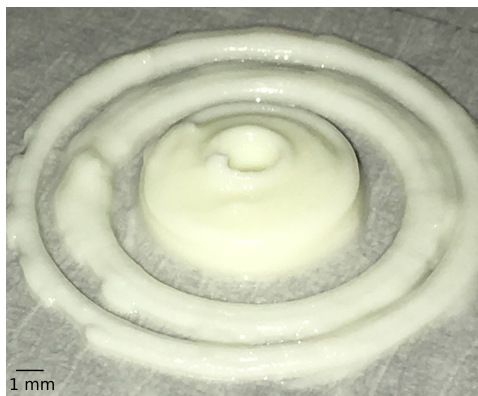
Figure 6.11: Concentric cylinders with skirt surrounding the print.
