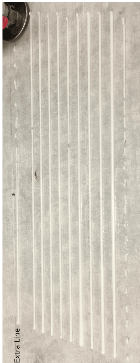
Figure 6.15: Test print to determine coasting settings.
