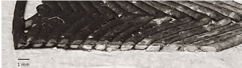
Figure 6.10: Visible gradient in cross section of print.
