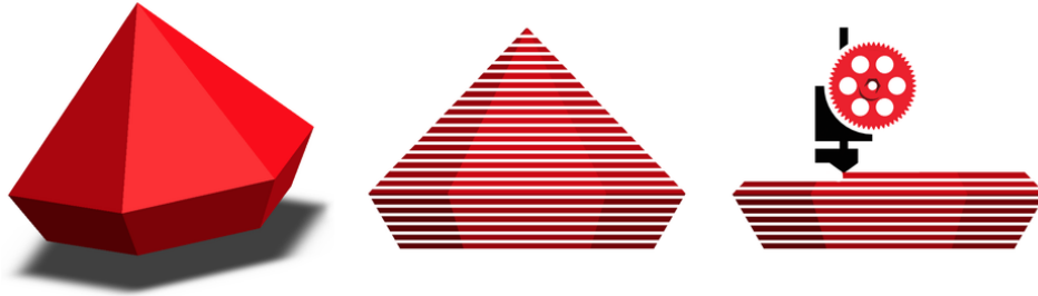
Figure 2.9: The general slicing and printing process.
