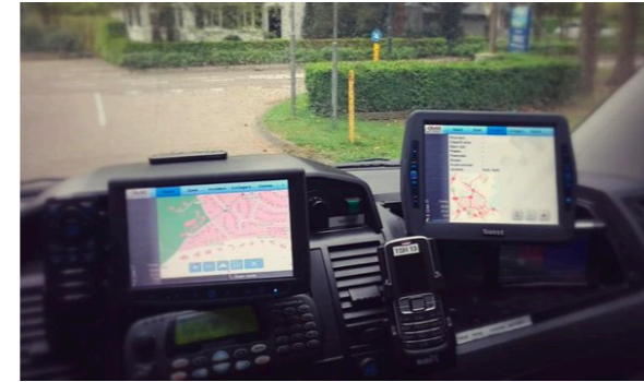
Figure 12. CityGIS; the ambulance staff receives the route and information typed by the reporting room employee via the CityGIS in the vehicle.
