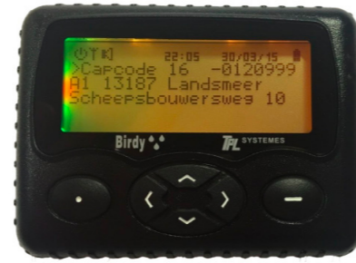
Figure 11. Pager; the ambulance staff receives first information from the reporting room via a pager.
