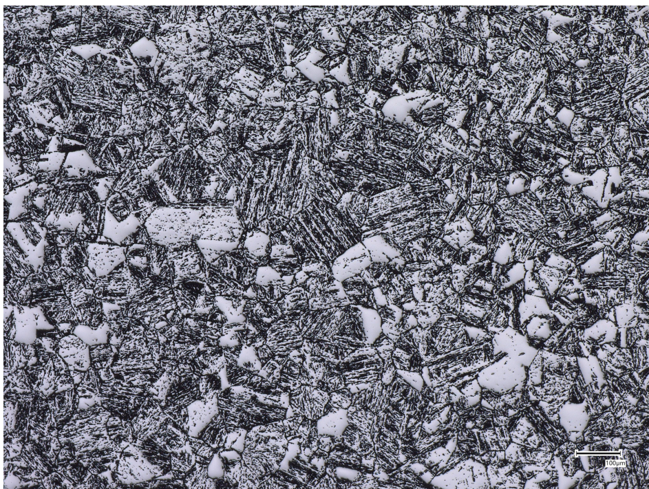
Fig 4.1. Optical microstructures revealed with chemical etching for (a) BASE; (b) LCLV and; (c) HCHV alloys, austenised for 5 minutes at 1100 °C and subsequently quenched.
