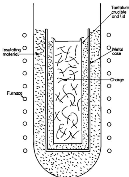
Figure 2.4 Experimental setup for the calciothermic reduction of REOs<sup>3</sup>
