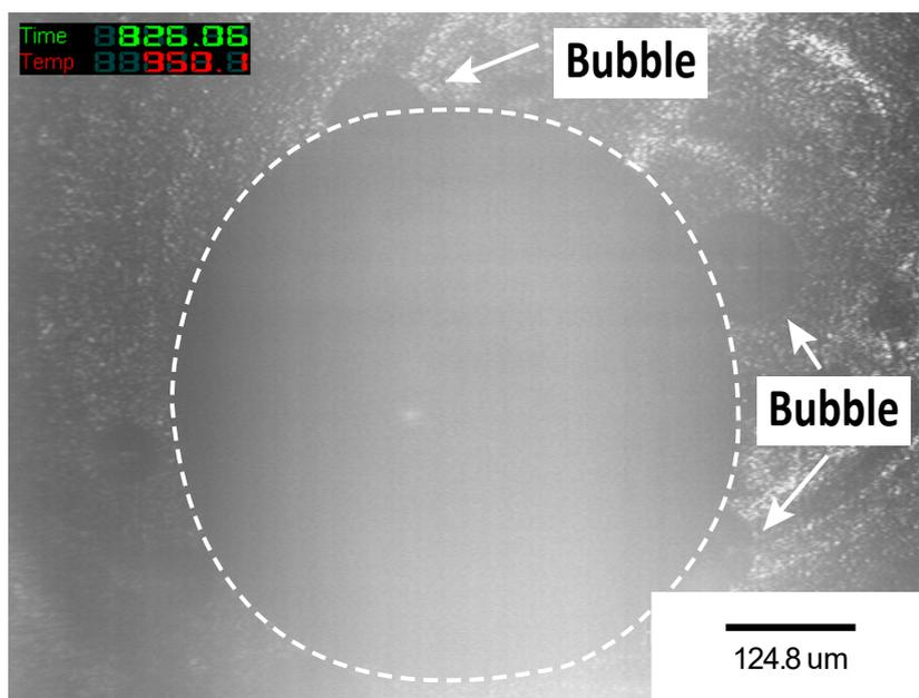
Figure 6.2 Release of bubbles during the dissolution of  $\text{Nd}_2\text{O}_3$  particles
