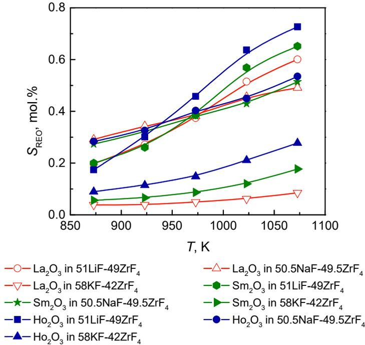
Figure 3.4 Solubility of lanthanide oxides in fluorozirconate melts (reproduced with data from reference <sup>21</sup>)
