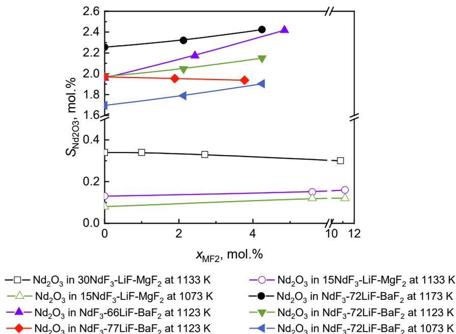
Figure 3.5 Solubility of  $Nd_2O_3$  in  $LiF-MF_2-NdF_3$  melts ( $M = Mg, Ba$ ) (reproduced with data from reference <sup>14,17</sup>)
