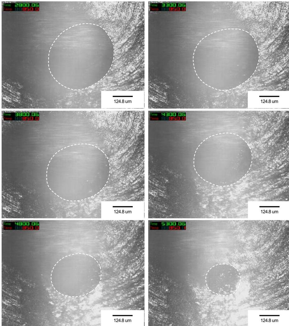
Figure 6.1 CSLM images of the dissolution of  $\text{Nd}_2\text{O}_3$  in  $\text{KF}\text{-}23\text{NdF}_3$  at 1141 K
