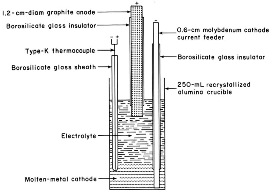
Figure 2.6 Electrolytic cell for recovery of REMs as alloys <sup>50</sup>
