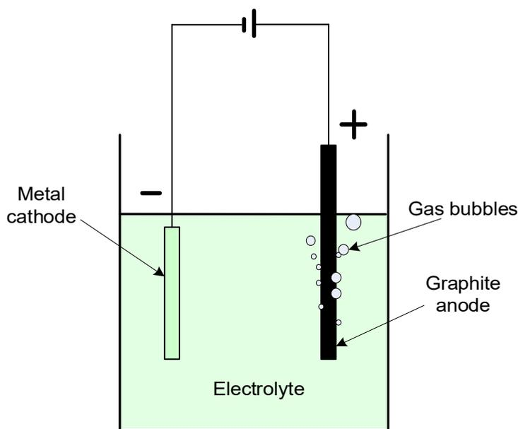
Figure 2.5 Cell construction of a typical electrolysis setup
