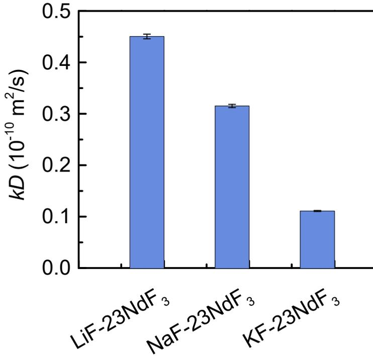
Figure 6.9 Influence of type of AF on  $\text{Nd}_2\text{O}_3$  dissolution in AF-23NdF<sub>3</sub> at 1141 K
