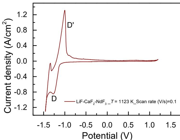
Figure 7.7 Cyclic voltammograms recorded on a molybdenum electrode in LiF-CaF<sub>2</sub>-NdF<sub>3</sub> at 1123 K melts with a scan rate of 0.1 V/s (vs. ref. Pt/PtO<sub>x</sub>/O<sup>2-</sup>)
