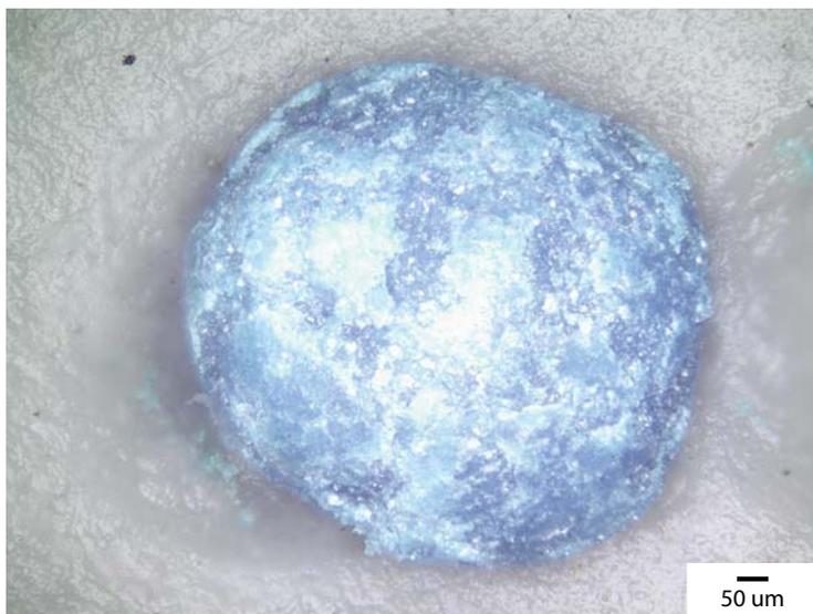
Figure 5.2 Quasi-spherical  $\text{Nd}_2\text{O}_3$  particle for CSLM experiments
