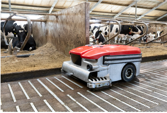
Figure 3: The Discovery Collector robot made by Lely, which is tasked to autonomously clean up all the manure in a cow barn. Source: [40]
