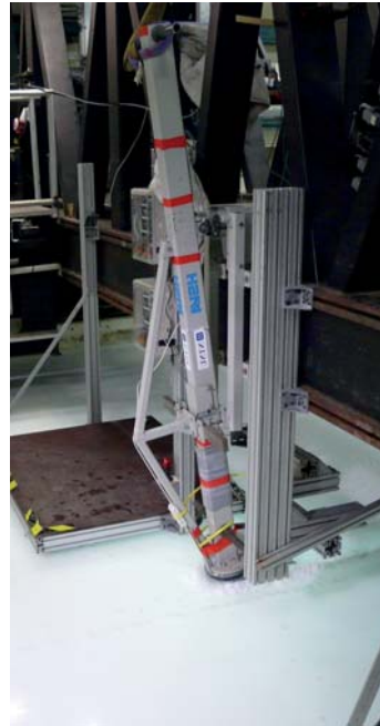
Figure 4.1: Test setup used in forced vibration experiments. The setup consisted of a vertical rigid beam with a cylindrical indenter at the ice level. An electric linear actuator was installed in order to control the motion of the structure. Displacements were measured by two lasers and the contact area, local pressures, and global ice load were measured by a tactile sensor. All measures are in mm.
