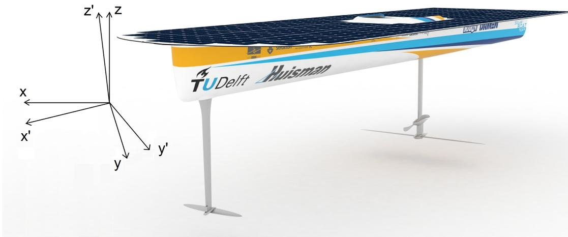
Figure 2.0.1: Earth- and body-fixed frames of reference
