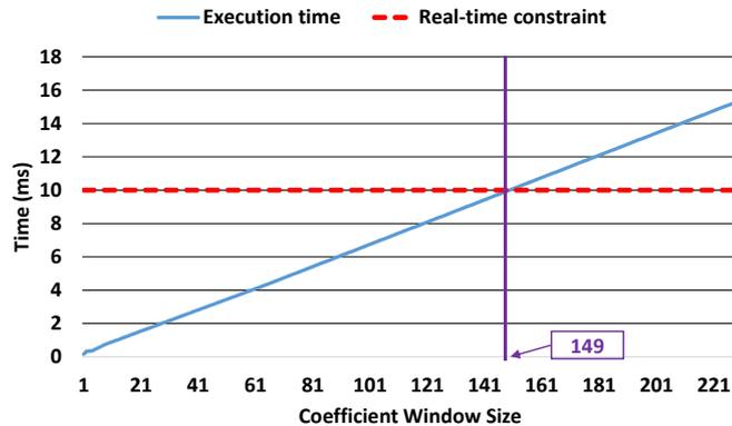
Figure 4.17: SiMS execution time for different window sizes for 20MHz clock frequency
