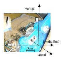
Fig. 3. Accelerometers mounted on the axle box in the vertical and longitudinal directions.
