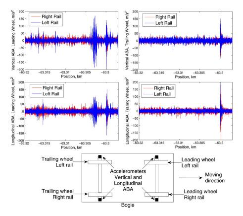
Fig. 10. Data obtained from the measurement system.
