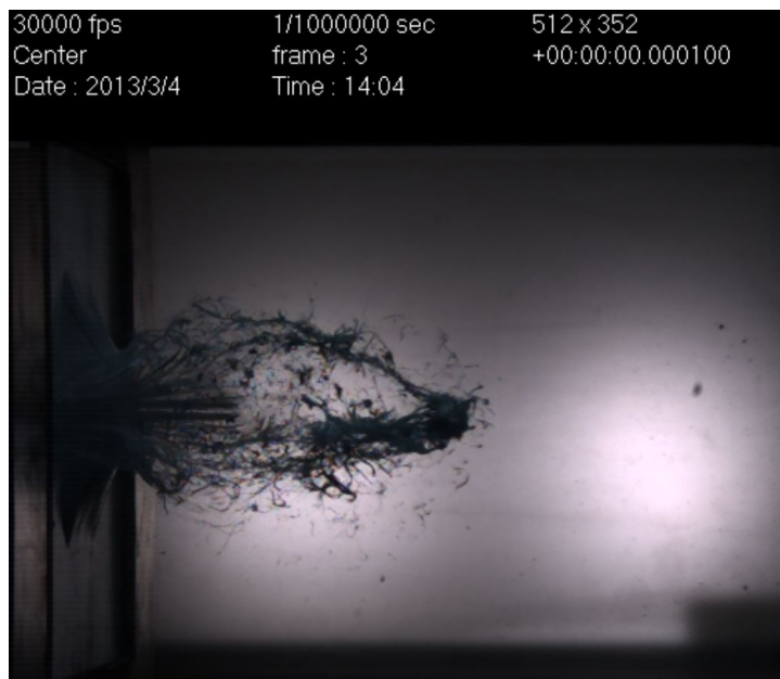
Figure 9.4: Experimental footage with V_0 = 3532 \text{ m/s} at t = 1.0 \cdot 10^{-1} \text{ ms} after impact [8].
