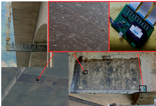
Fig. 33. Smart film used on Taipingzhuang bridge (taken from [101]).
