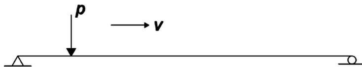
Figure 4.1: Moving load model
