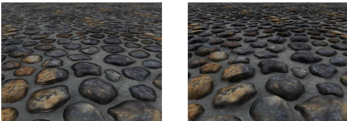
Figure 8. Simple parallax mapping (left) vs. parallax occlusion mapping (right).
