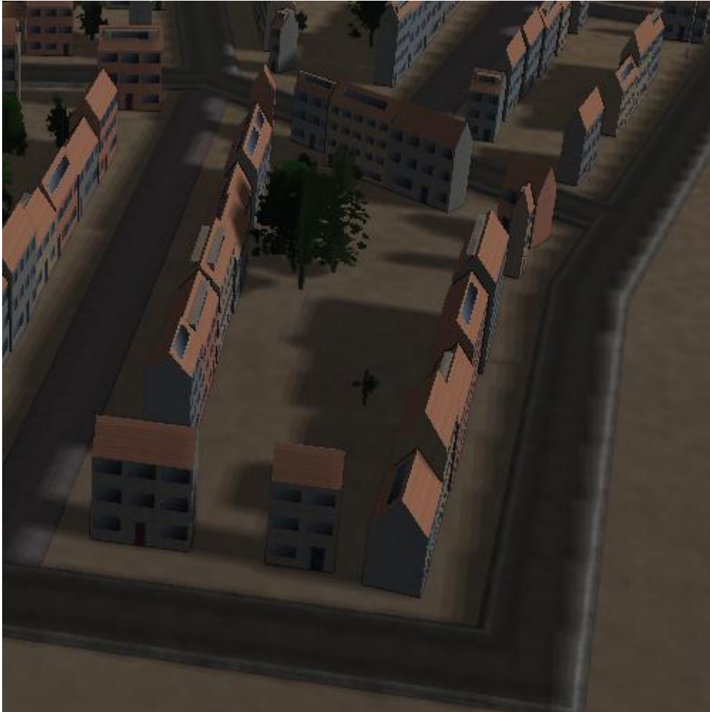
Figure 16. Due to insufficient precision, the road casts shadows on itself.
