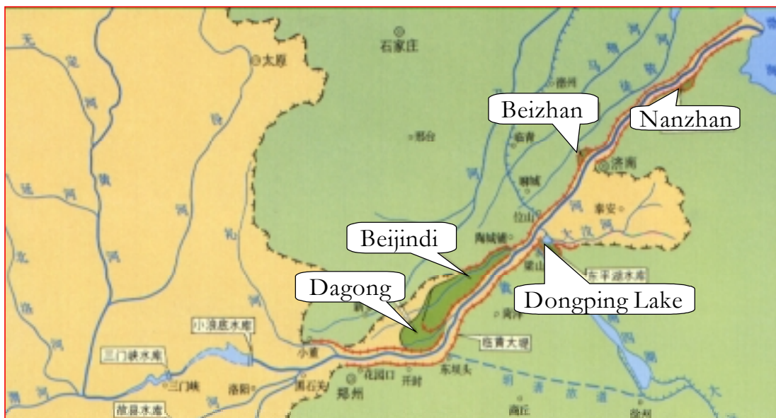
Figure 18: The five detention basins in the lower reach (Source: YRCC, 2001)
