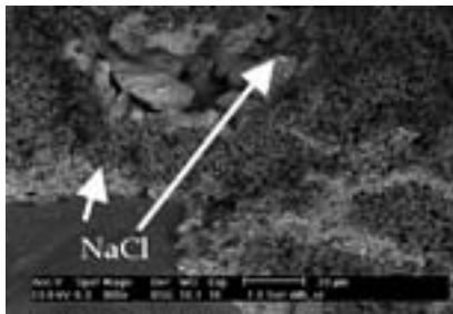
Figure 12: ESEM photomicrographs showing NaCl (lighter areas) crystallizing as a layer over the pore walls of the binder
