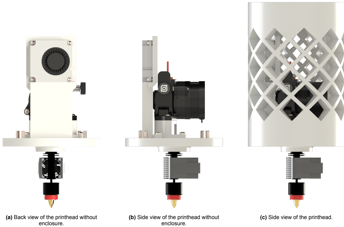
Figure 3.3: Several renders of the custom designed printhead.
