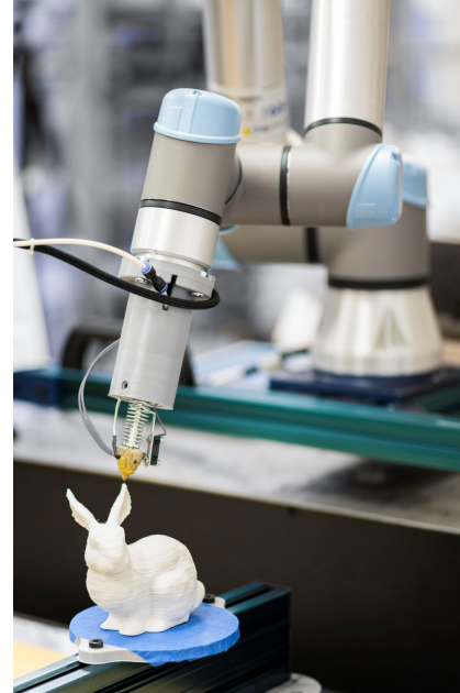
(b) Printed result of one of the S^3 -Slicer toolpaths [20].
