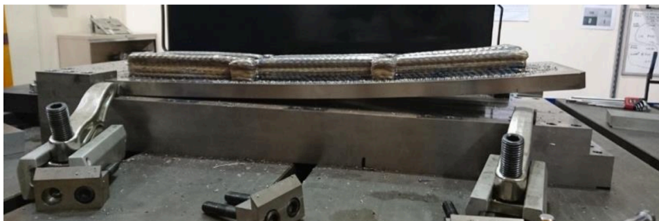
Figure 1.1: Deformation after unclamping an object manufactured with WAAM [7].
