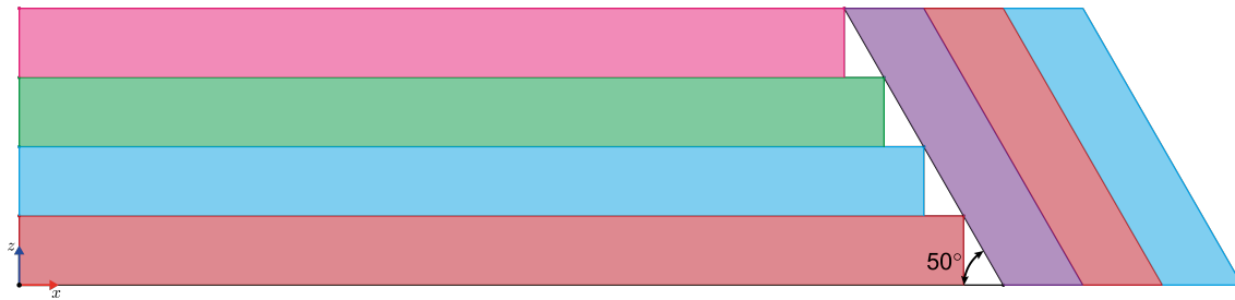
Figure 4.5: Toolpath around the incline for the global slope test.
