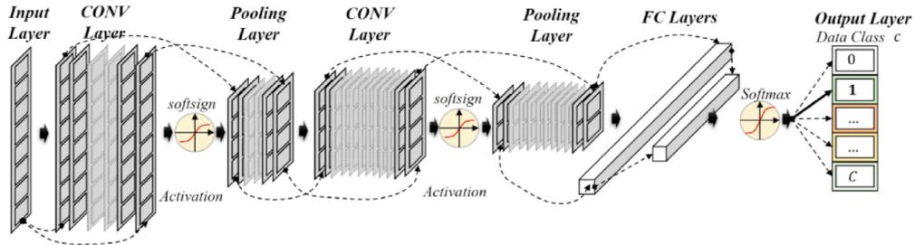
Figure 2.3.: Illustration of CNN structure for a data classification task [41]
