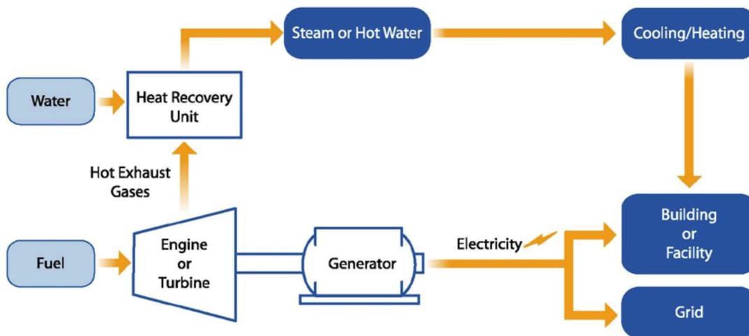
Figure 3.3.: Diagram of a CHP Installation
