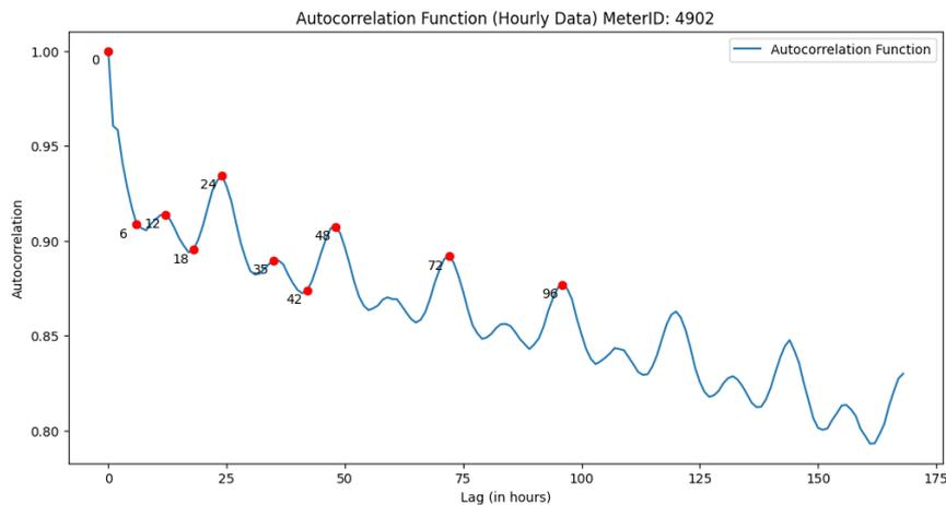
Figure 5.5.: Autocorrelation of Hourly Consumption of Meter ID 4902
