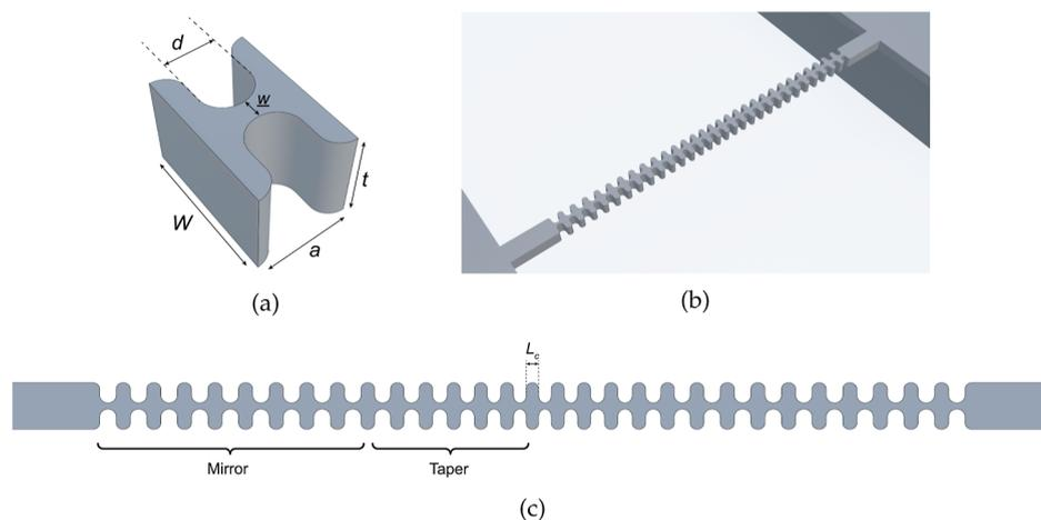
**Figure 5.** A visual representation of the geometric properties of the base design for the fishbone nanobeam cavity. (a) A 3D model of the corrugated unit cell, highlighting its key design parameters. (b) A 3D model of the complete fishbone nanobeam cavity. (c) A 2D schematic of the fishbone nanobeam cavity, highlighting the mirror, taper and cavity region.
