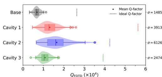
**Figure 8.** Box plots overlaid with violin plots show the  $Q$ -factor distributions for fishbone base (black), cavity 1 (red), cavity 2 (blue), and cavity 3 (green) across different surface roughness configurations. A dotted line indicates the  $Q$ -factor for each structure under ideal (no surface roughness) conditions. The standard deviation ( $\sigma$ ) of each distribution is provided on the right.
