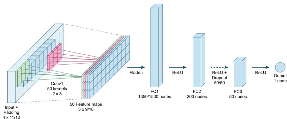
**Figure 2.** A schematic representation of the CNN architecture employed to optimize nanobeam cavities for fabrication error tolerance. The CNN consists of a convolutional layer followed by three FC layers, with dropout applied between the second and third FC layers to reduce overfitting. Zero-padding is applied to the input, and the ReLU activation function is utilized.<sup>37,38</sup>
