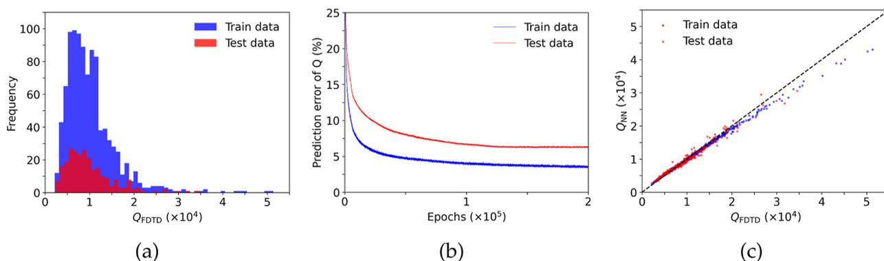
**Figure 3.** An overview showcasing an example of the data set, training, and correlation plots for L2 nanobeam cavities under ideal conditions, trained without  $L^2$ -regularization. Additional plots are provided in the Appendix. (a) Data set split before preprocessing. (b) Prediction error progression during training. (c) Correlation between predicted  $Q$ -factors ( $Q_{NN}$ ) and simulated  $Q$ -factors ( $Q_{FDTD}$ ).
