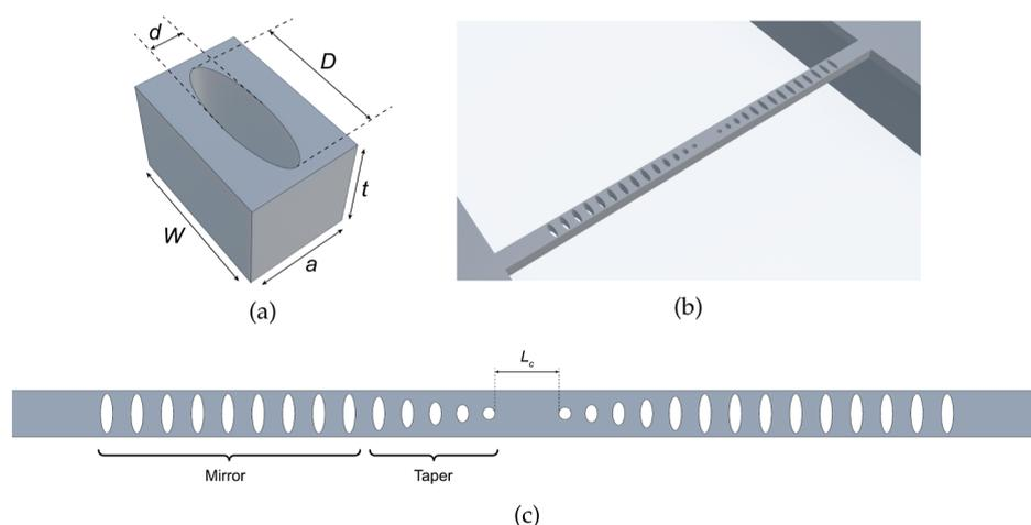
**Figure 4.** A visual representation of the geometric properties of the base design for the L2 nanobeam cavity. (a) A 3D model of the elliptical airhole unit cell, highlighting its key design parameters. (b) A 3D model of the complete L2 nanobeam cavity. (c) A 2D schematic of the L2 nanobeam cavity, highlighting the mirror, taper and cavity region.
