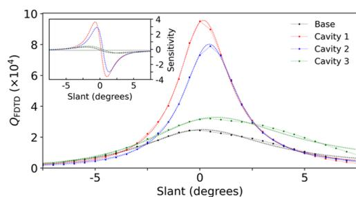
**Figure 9.** A graph showing the  $Q$ -factor of L2 base (black), cavity 1 (red), cavity 2 (blue), and cavity 3 (green) as a function of slant angles. The data is fitted with a linearly asymmetric Lorentzian curve, and its derivative, displayed in the inset, quantifies the sensitivity of the  $Q$ -factor to slant angle variations in units of  $\times 10^4/\text{degree}$ .
