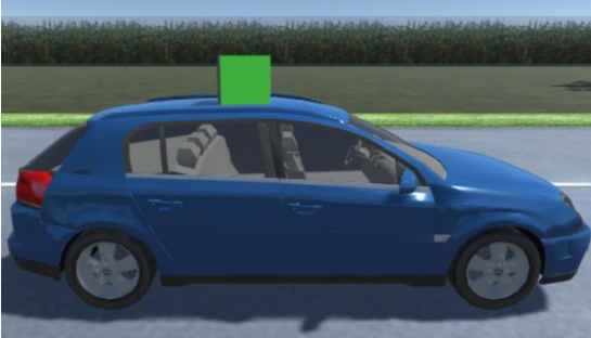
Figure 1: AV with an eHMI in the form of a cube. The eHMI exhibits green to signal HDVs to cross.
