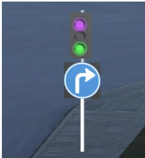
Figure 44: Signalling device expresses intent of automated vehicle to drive first (purple), and second (green) at intersection.
