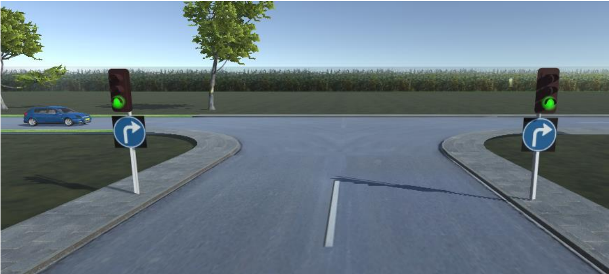
Figure 16: eHMI on the infrastructure where signals communicate AV intent. For instance, AV requests the HDV to cross first through a green signal.
