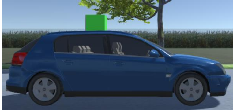
Figure 43: Automated vehicle with the absence of human in the driver seat. A light display on top of vehicle expresses vehicle intent to drive first (purple), or second (green) at intersection.
