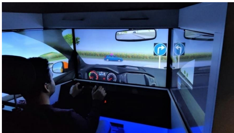
Figure 11: Participant driving in a fixed-base simulator.
