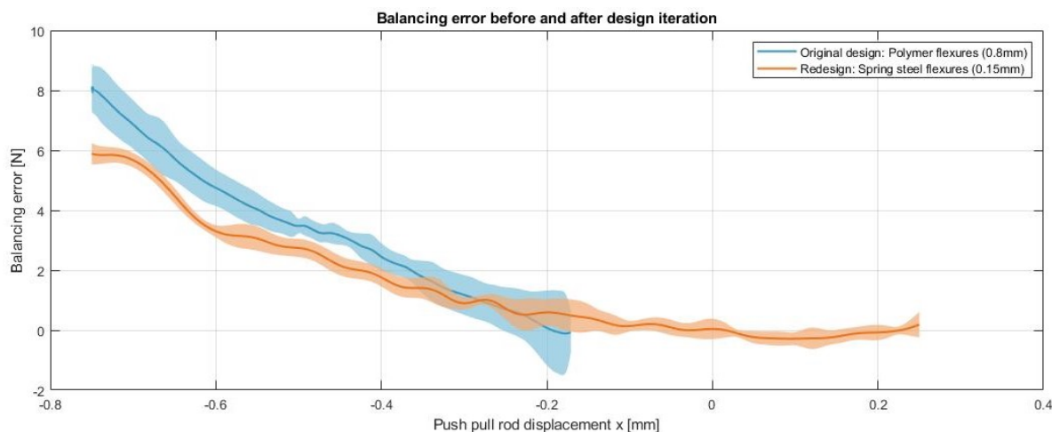
Figure 8.6: Balancing error F_{err} (mean and SD, n = 6 ) before and after replacing the handle flexures, showing mean and standard deviation. Again, x = 0\text{mm} at the neutral state and x = -0.75\text{mm} at the closed state. This figure contains results from both Paragraph 8.3 and 8.4.
