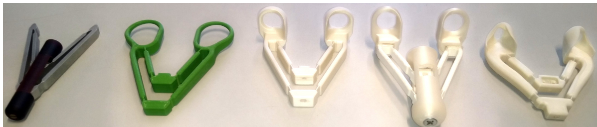
Figure 7.6: Mock-up tweezers handles 3D-printed during the final design phase showing handle design evolution, with the final design on the right.
