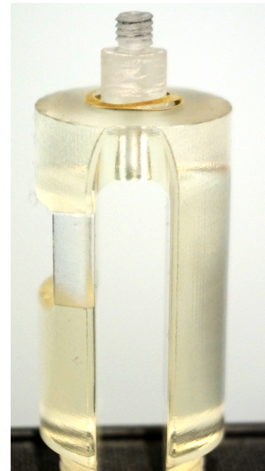
Figure 8.4: Location of the cupped spring washers that prevent longitudinal hysteresis.
