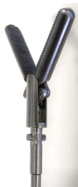
Figure 1.1: Typical laparoscopic grasper tip, with links and joints causing friction, play and hysteresis.
