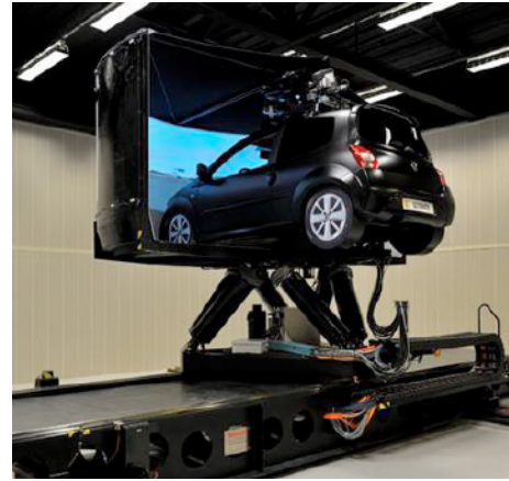
(b) 8 DOF Renault ULTIMATE motion platform [3]
