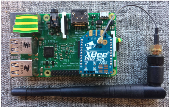
(a) The Raspberry Pi 3B connected to a XBee module
