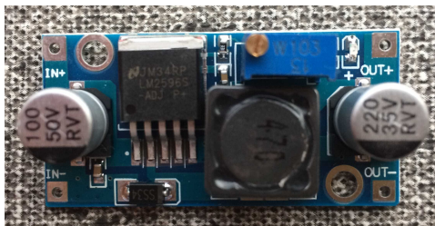
(a) The LM2596S buck converter
