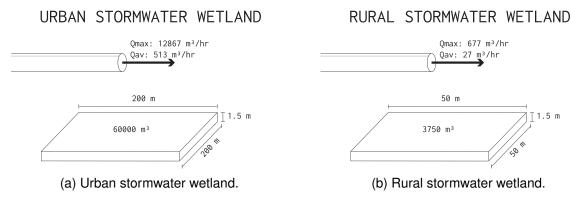
Figure 19: Wetland design, recharged with stormwater.
