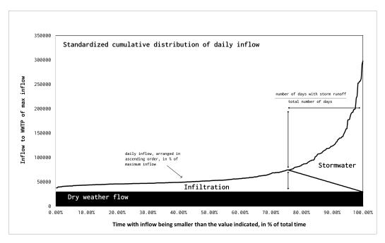
Figure 10: Determination of average dry weather flow, stormwater and infiltration by the "triangle method" in volume.
