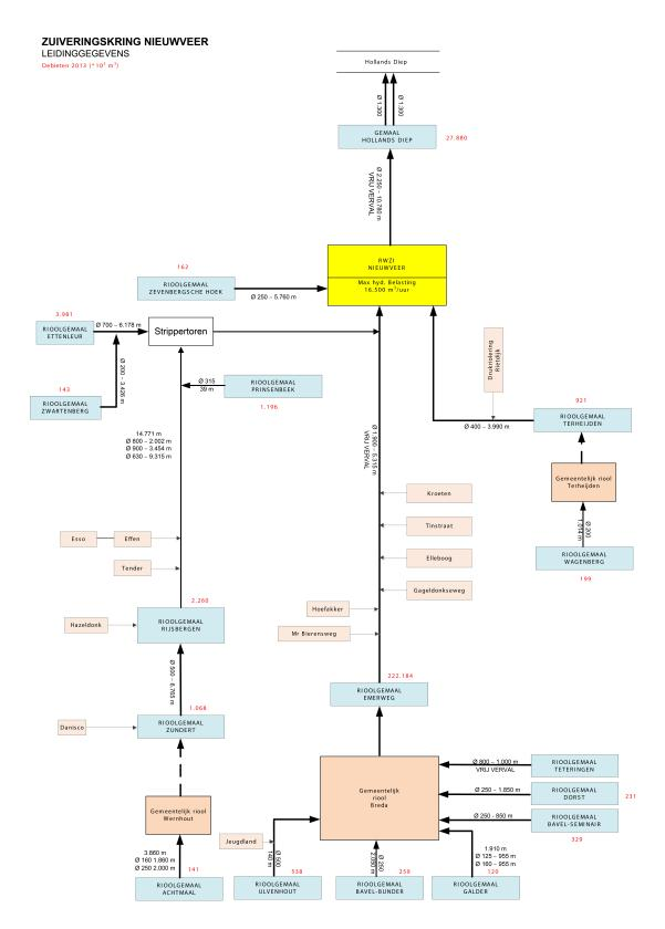
Figure 8: Nieuwveer wastewater treatment plant scheme for 2013. Written in red the annual flow in  $10^3 \ m^3$ .[65]
