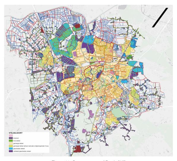
Figure 11: Sewer system of Breda.[65]
