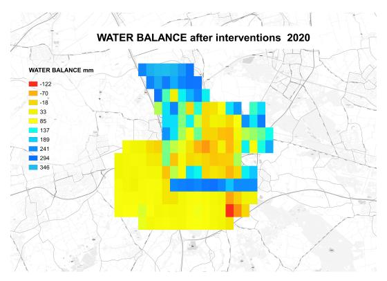
Figure 23: Representation of the annual water balance for the municipality of Breda, through QGIS 3.10, after the application of the final strategy.
