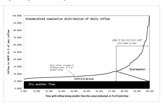
Figure 9: Determination of average dry weather flow, stormwater and infiltration by the "triangle method" in %.
