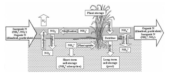
Figure 13: Nitrification cycle in a constructed wetland [156].
