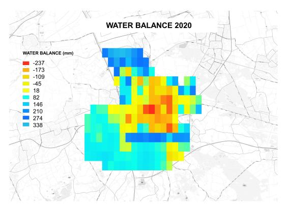
Figure 22: Representation of the annual water balance for the municipality of Breda, through QGIS 3.10., before thje application of the final strategy.
