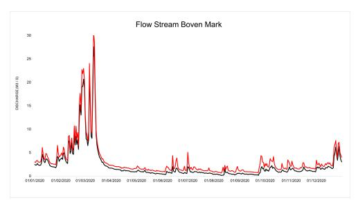
Figure 14: Boven Mark flowrate. In black flowrate of 2020, in red river flowrate increased by wastewater effluent [65].
