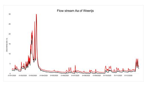
Figure 15: Aa of Weerijs flowrate. In black flowrate of 2020, in red river flowrate increased by wastewater effluent [65].
