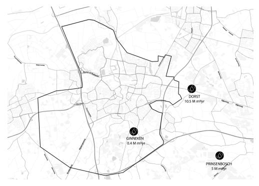
Figure 7: Extraction groundwater area for Breda's municipality. [64]
