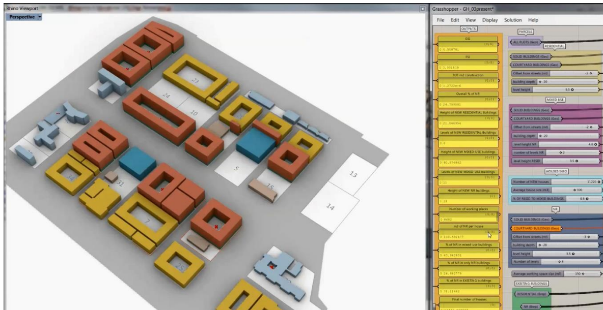
Figure 35. Interface of the tool. Left - 3D visualization in the Rhino viewport. Right - GH window with info panels and data nodes.
