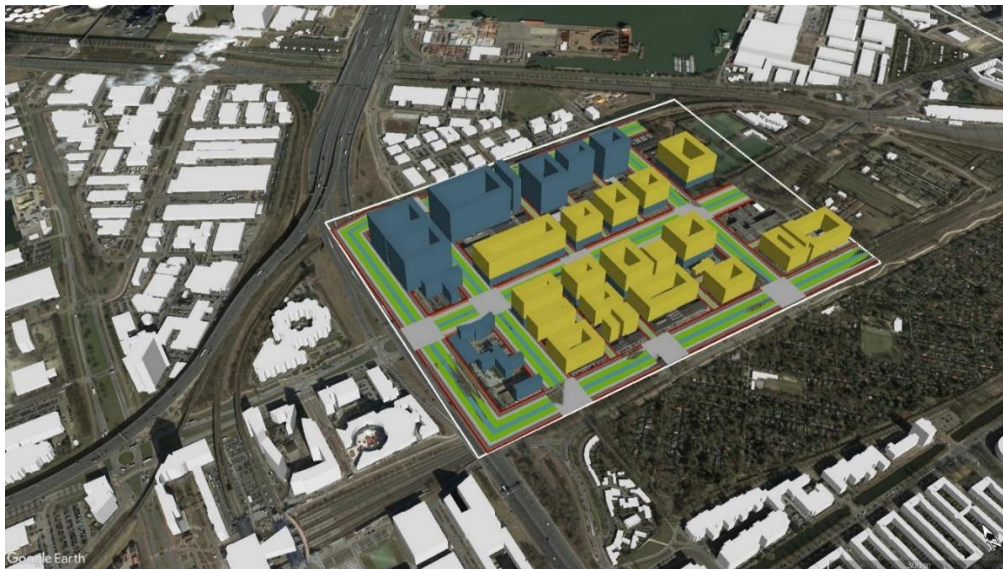
Figure 56. Visualization of a CityGML model from a proposal loaded into Google Earth (G. Aguiaro).
