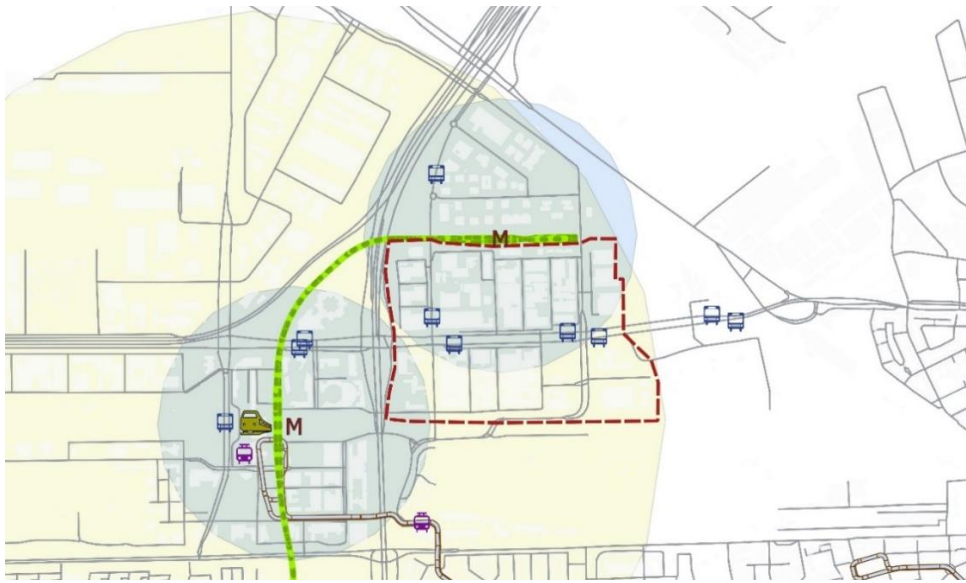
Figure 49. Extract from the QGIS map. The yellow circle is the 1500-meter radius from the train station and the blue circles the 500-meter radius from the metro stations. The red dashed line is Sloterdijk One.
