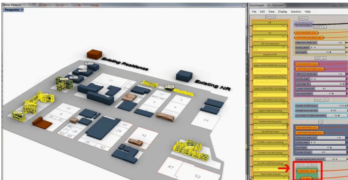
Figure 37. Highlighted in red, the existing building nodes to select the buildings to keep.
