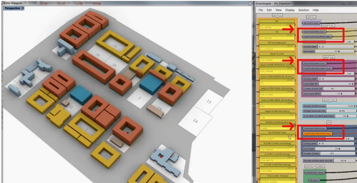
Figure 38. Highlighted in red, the nodes of courtyard and solid buildings to select the plots to create buildings.
