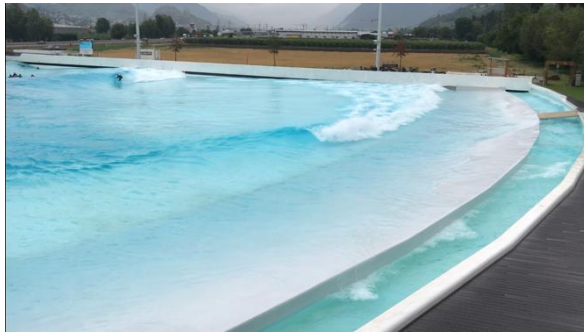
(a) First time instant: the broken wave propagates towards the edge. A minor wave height decay between the first wave and the second wave (with the surfer). The water level at the slope of the edge and in the gutter can be seen to be located at the still water level. The water in the gutter is relatively calm.
