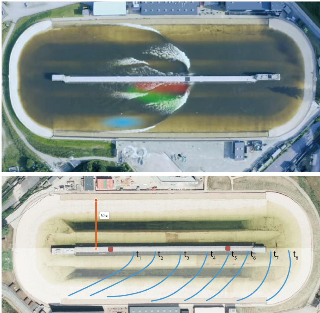
Figure 2.35: Analysis of the wave crests evolution and refraction at the Surf Snowdonia wavepool in Wales (Maps, n.d.).
