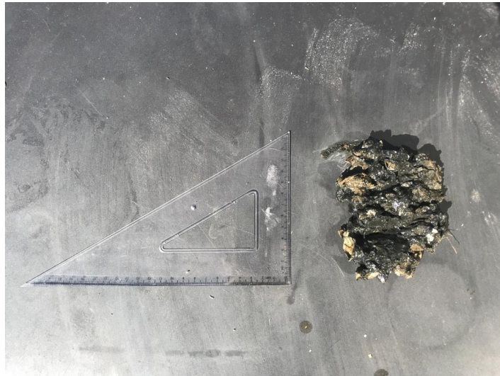
Figure 3.10: Sediment sample 3: Mud mixed with shells
