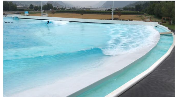
(b) Second time instant: it can be seen that the broken wave runs-up the edge, just before the wave overtops the edge. A certain section of the wave is still unbroken as it runs-up the slope of the edge. The water level in the gutter is not affected yet by the wave run-up.
