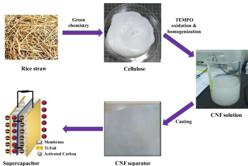
Figure 3. Schematic representation of the preparation of the supercapacitor. The membrane used as a separator is made by casting a mixture of cellulose nanofibrils and distilled water onto a PTFE plate. The Figure was obtained by kind permission from [20].
